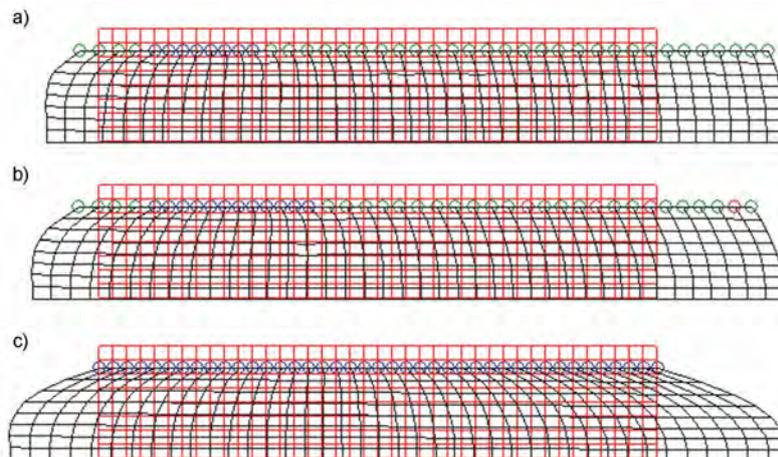
Fig. 8. The ring deformation for deflection  $f = 1.5$  mm and various friction coefficients which were taken into calculations: a)  $\mu = 0.3$ , b)  $\mu = 0.6$ , c)  $\mu = \infty$
