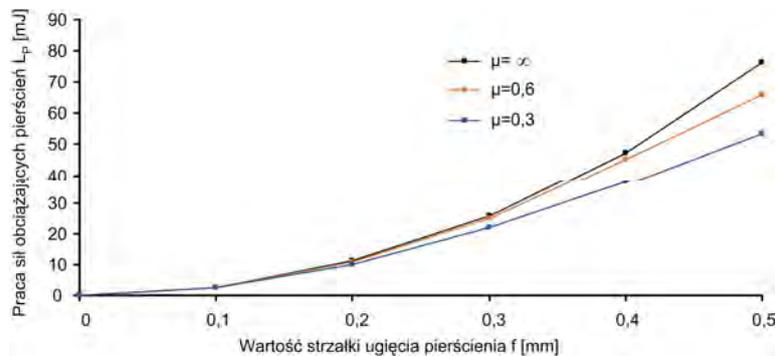
Fig. 5. The work of ring load in relation to its deflection
