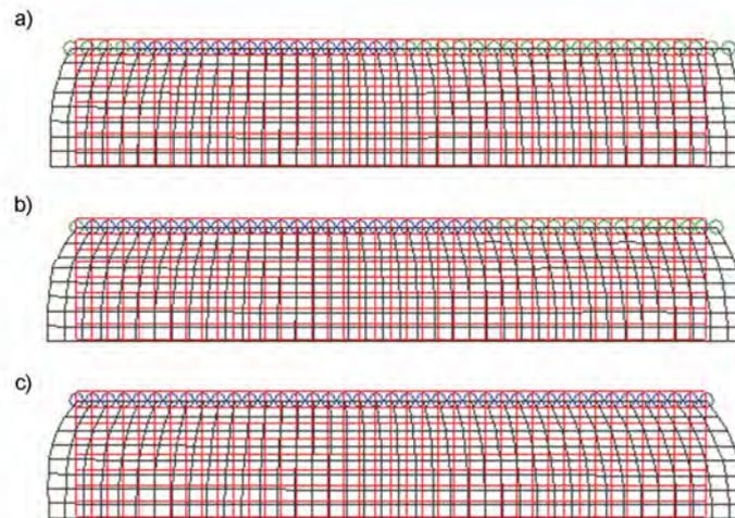
Fig. 4. The ring deformation for deflection  $f = 0.5$  mm and various friction coefficients which were taken into calculations : a)  $\mu = 0.3$ , b)  $\mu = 0.6$ , c)  $\mu = \infty$
