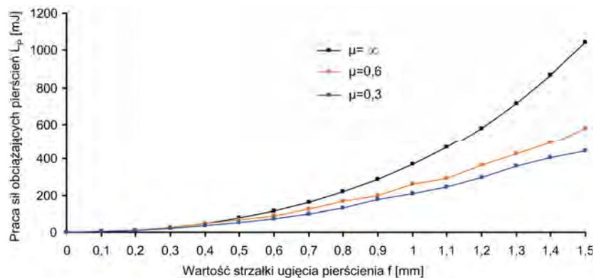
Fig. 9. The work of ring load in relation to its deflection
