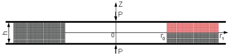
Fig. 3. The rubber ring division into finite elements
