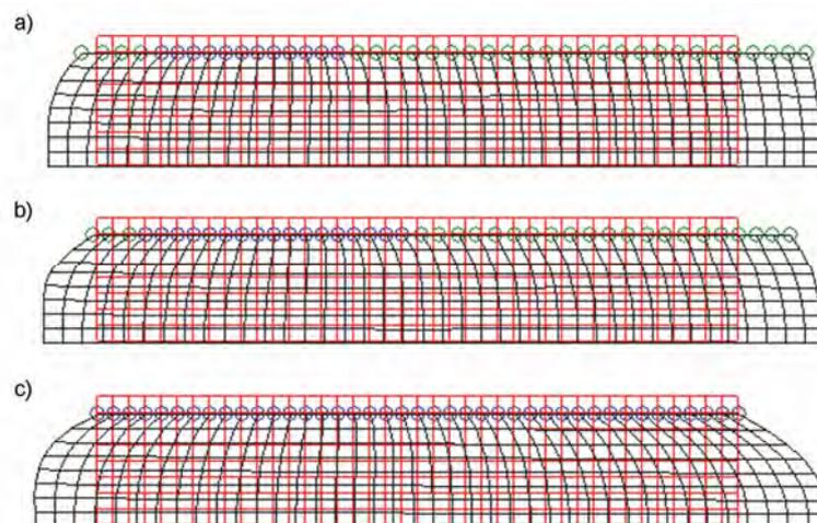
Fig. 6. The ring deformation for deflection  $f = 1$  mm and various friction coefficients which were taken into calculations: a)  $\mu = 0.3$ , b)  $\mu = 0.6$ , c)  $\mu = \infty$
