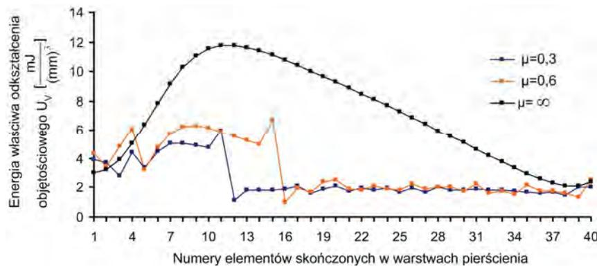
Fig. 11. Distribution of volumetric strain energy density in the surface layer under plate
