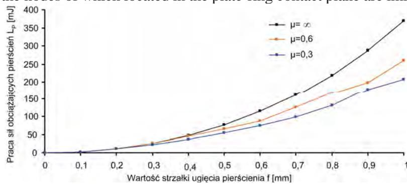
Fig. 7. The work of ring load in relation to its deflection
