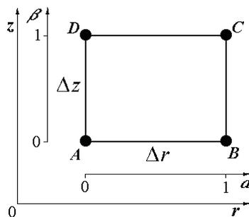
Fig. 1. Axisymmetrical finite element in a ring shape with rectangular cross-section and nodes in points A, B, C, D
