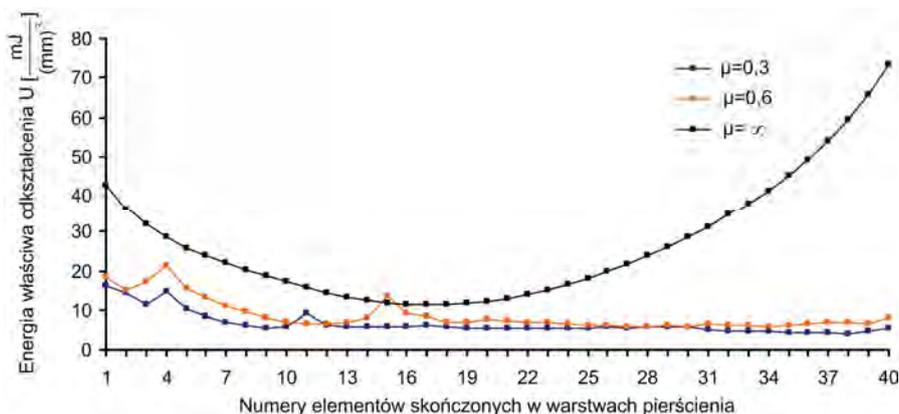
Fig. 12. Distribution of strain energy density in the surface layer under plate
