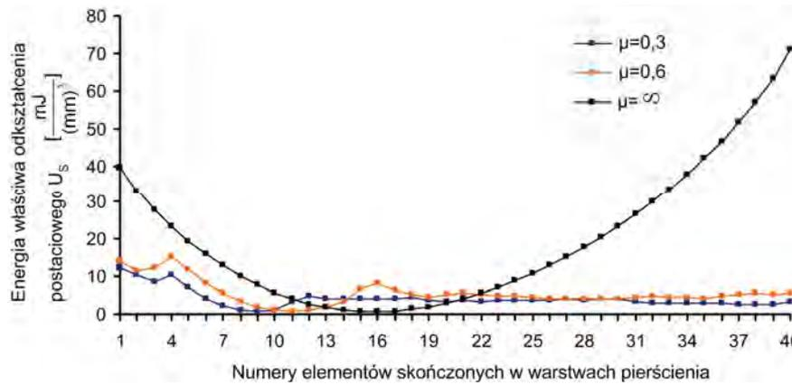
Fig. 10. Distribution of deviatoric strain energy density in the surface layer under plate
