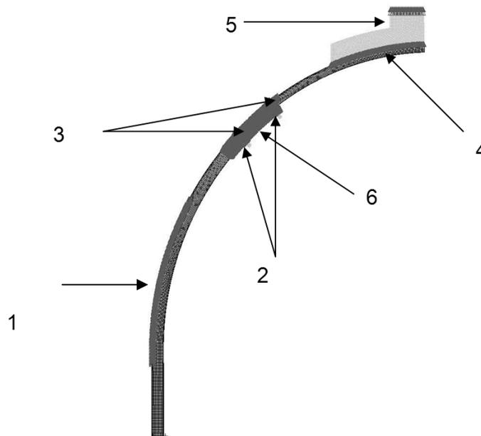
Fig. 11. Computational model of yielding arch support
