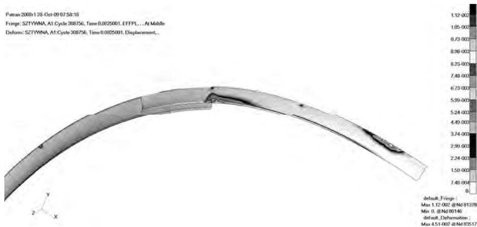
Fig. 6. Map of plastic deformation of part of LP8\_v25 arch support
