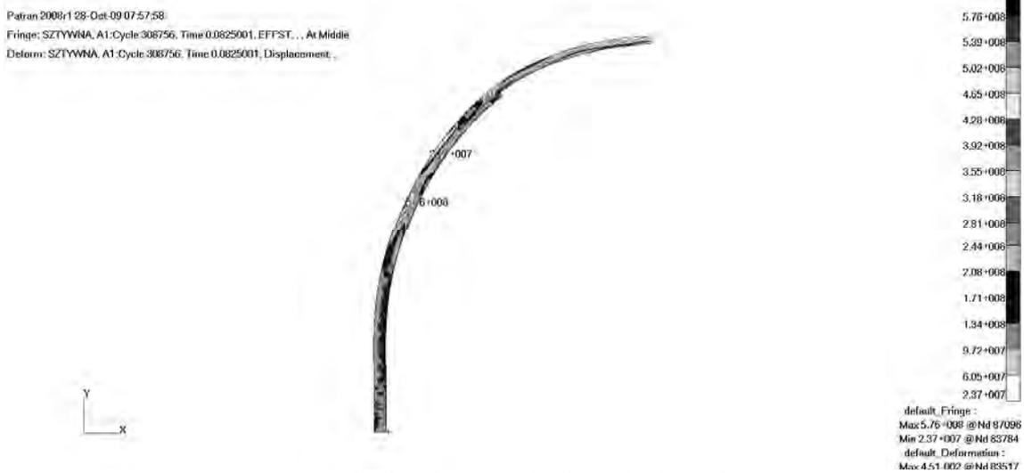
Fig. 5. Map of reduced stresses for the LP8\_v25 arch support
