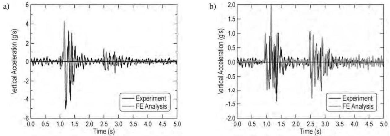
Fig. 9. Comparison between time histories of the vertical acceleration obtained from the experimental tests and FE analysis for the rear tandem axles of the truck tractor (velocity of 24 km/h): rear tandem axle (a), point located on the frame above the rear tandem axles close to the fifth wheel (b)
