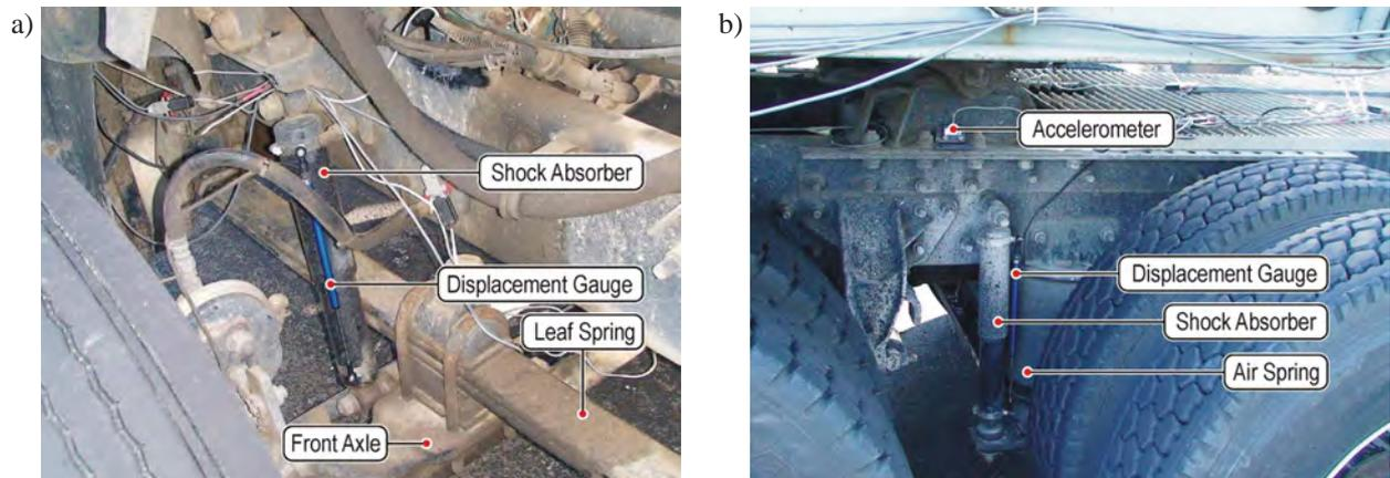
Fig. 2. Location of the displacement gauges and the accelerometers for the truck tractor: front steer axle (a), forward drive tandem axle (b)
