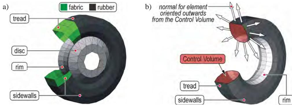
Fig. 6. FE model of the wheel (a) and components used in the airbag model (b)
