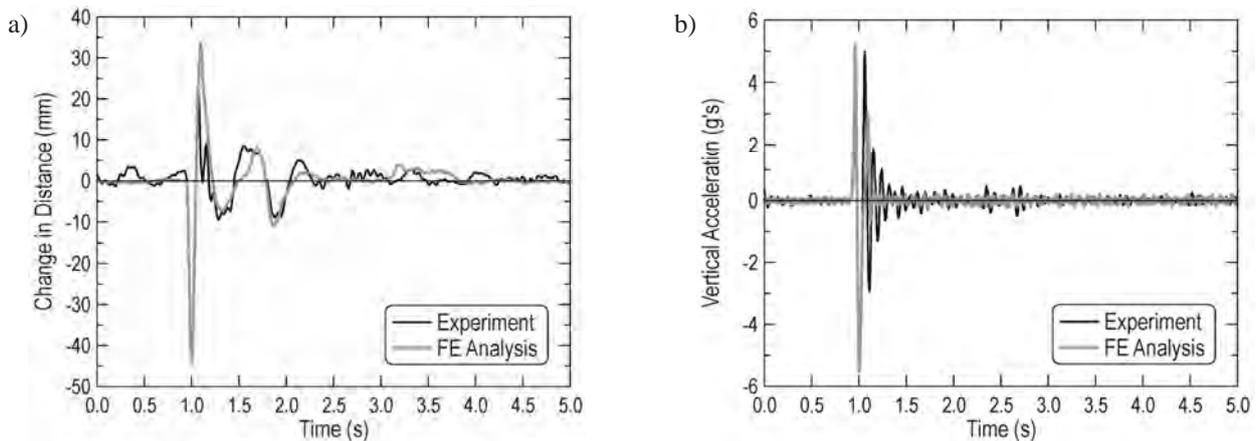
Fig. 7. Comparison between time histories obtained from the experimental tests and FE analysis for the front axle of the truck tractor (velocity of 24 km/h): change in distance between axle and frame (a), vertical acceleration of the axle (b)
