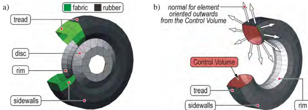
Fig. 6. FE model of the wheel (a) and components used in the airbag model (b)
