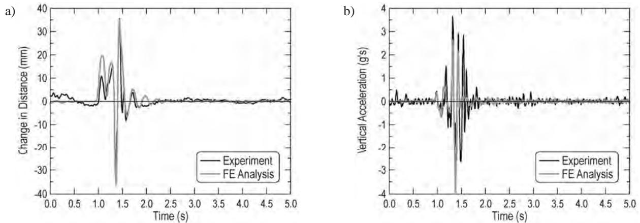
Fig. 10. Comparison between time histories obtained from the experimental tests and FE analysis for the third trailer axle (velocity of 24 km/h): change in distance between axle and the load deck (a), vertical acceleration of the axle (b)
