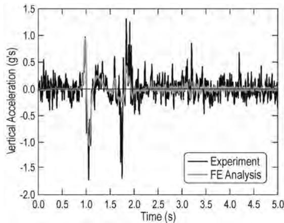
Fig. 8. Comparison between time histories of vertical acceleration obtained from the experimental tests and FE analysis for points located on the frame above the front axle of the truck tractor (velocity of 24 km/h)
