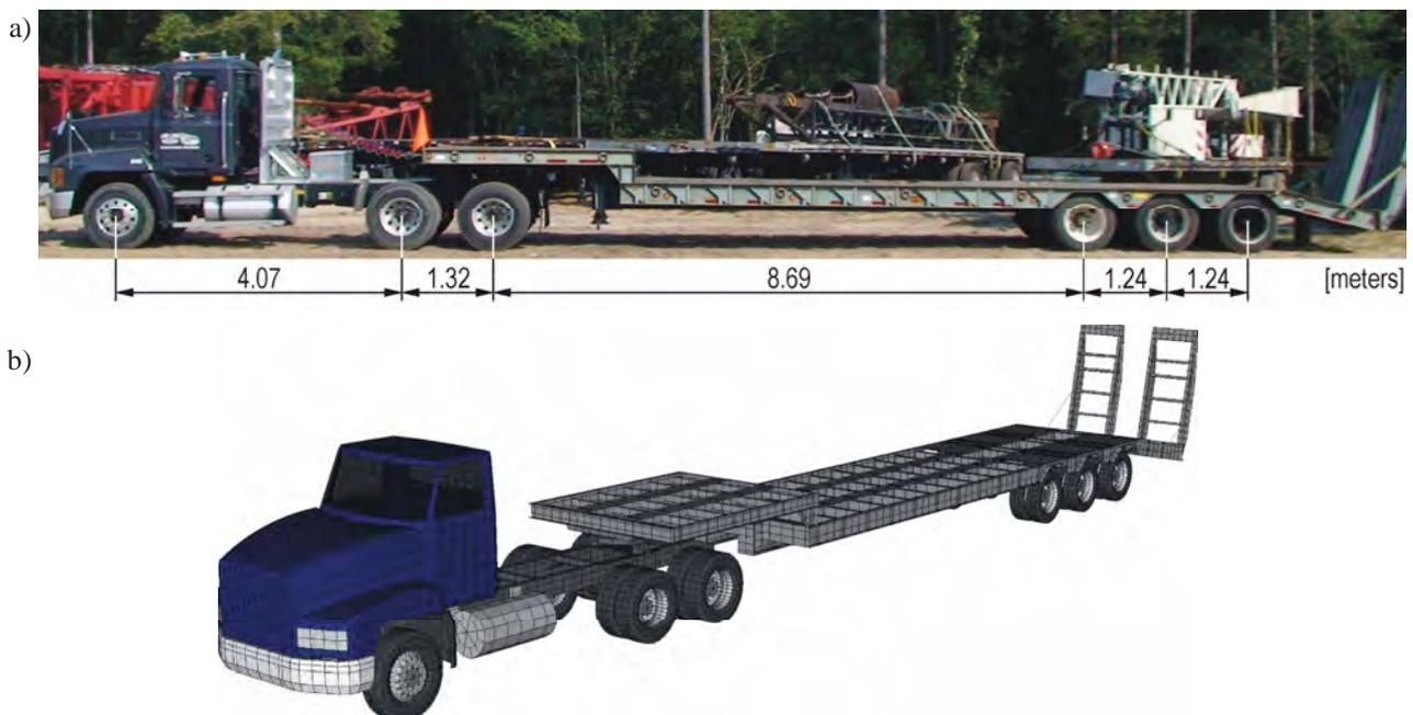
Fig. 3. The heavy vehicle selected for the tests (a) and its FE model (b)
