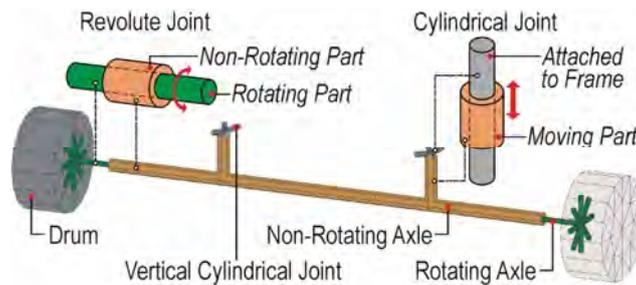
Fig. 4. Scheme of constrained joints applied in the FE model of the front suspension system
