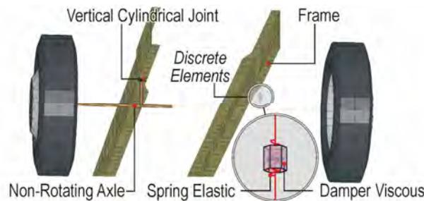
Fig. 5. Discrete elements in the FE model of the front suspension system
