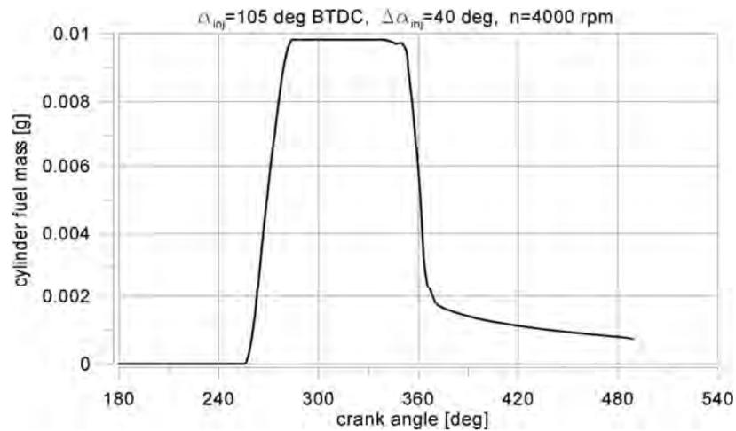
Fig. 4. Mass of CNG in the cylinder for injection fuel dose equal to 0,0098 g/cycle at 4000 rpm
