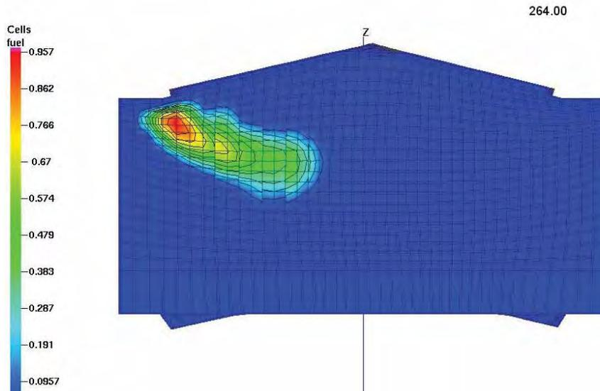
Fig. 7. Distribution of CNG during injection at 96° BTDC with injector to cylinder axis inclination angle of 70°
