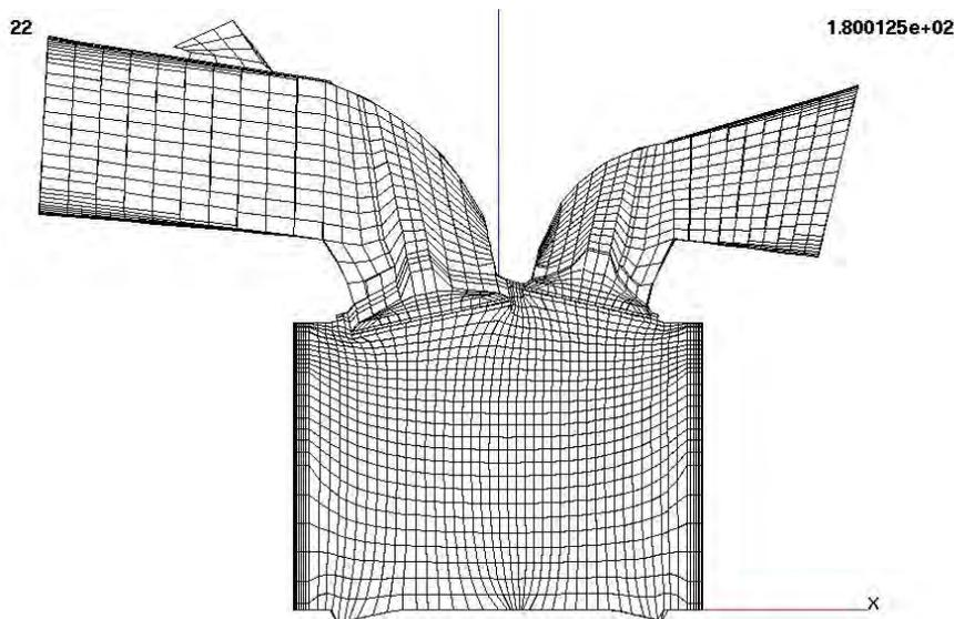
Fig. 3. Cross-section through the valves on calculation mesh of motorcycle engine SUZUKI DR-Z400S
