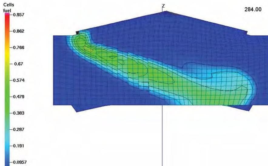
Fig. 8. Distribution of CNG during injection at 76° BTDC with injector to cylinder axis inclination angle of 70°
