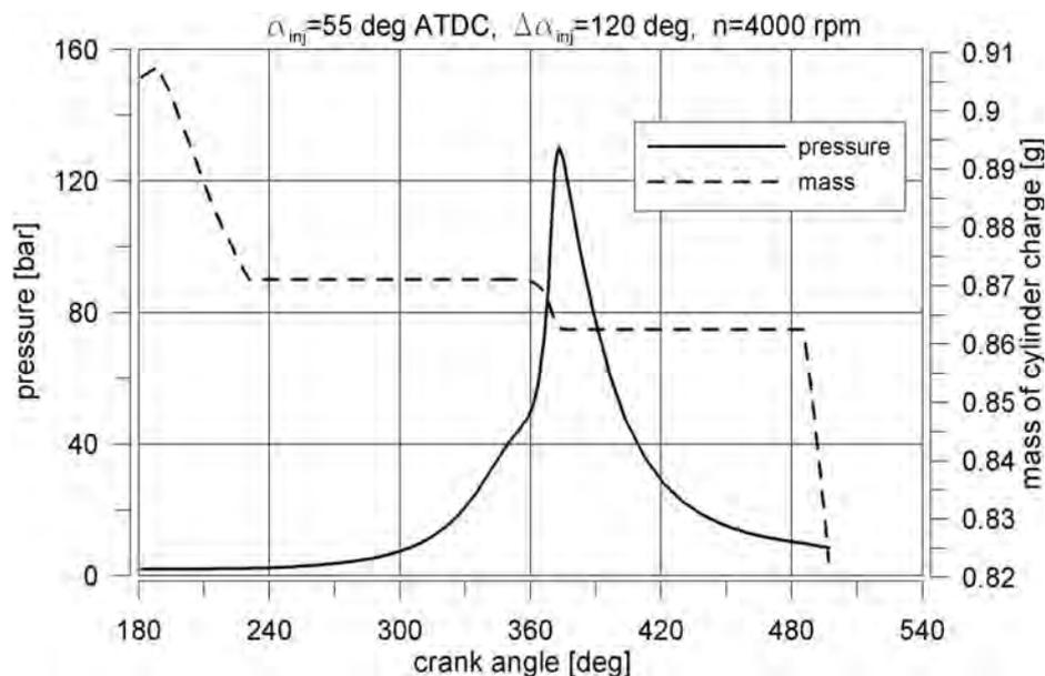
Fig. 10. Cylinder pressure and charge mass in the high-charged engine working at homogenous charge mode
