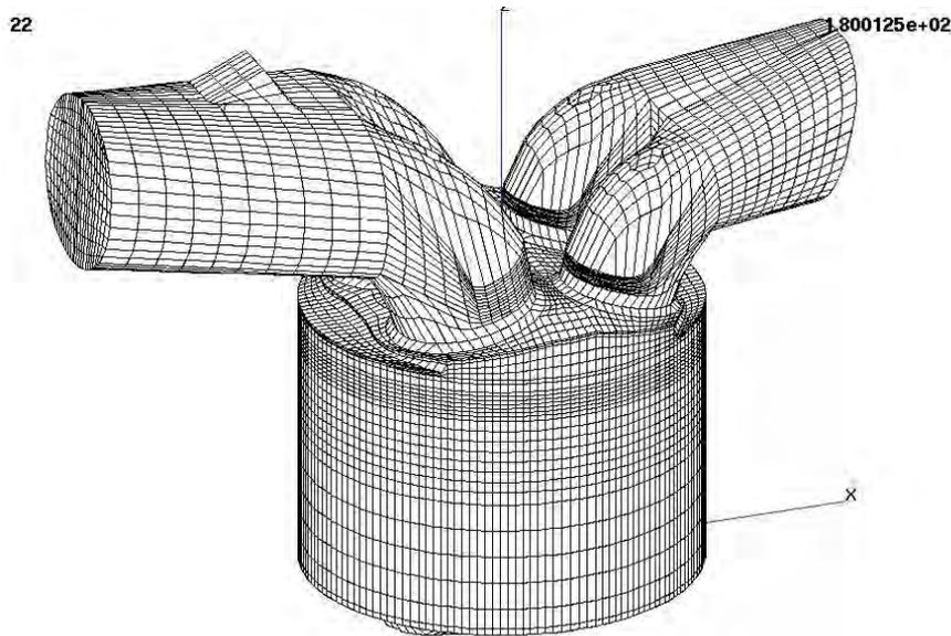
Fig. 2. Calculation mesh of motorcycle engine SUZUKI DR-Z400S
