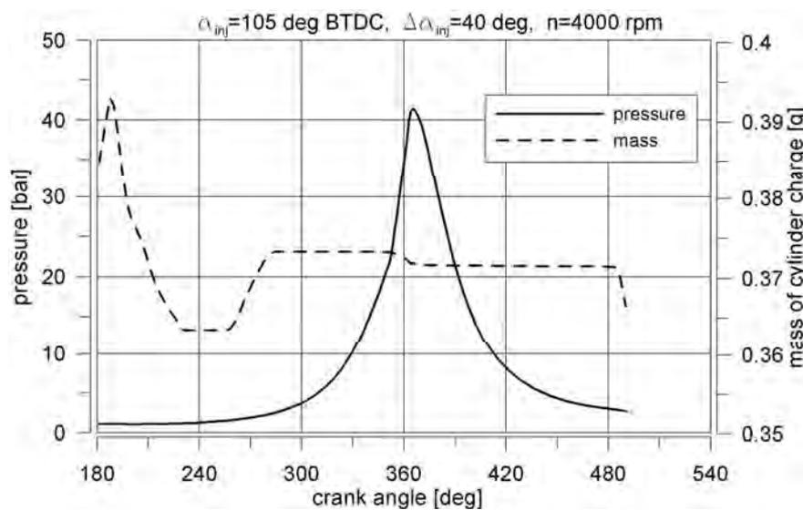
Fig. 9. Cylinder pressure and charge mass in the naturally aspirated engine working in stratified charge mode
