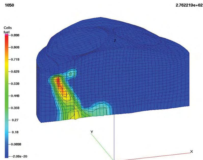
Fig. 5. Distribution of CNG during injection at  $84^\circ$  BTDC with injector to cylinder axis inclination angle of  $26^\circ$
