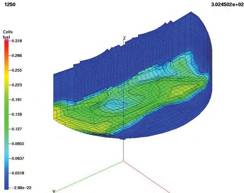
Fig. 6. Distribution of CNG during injection at 58° BTDC with injector to cylinder axis inclination angle of 26°
