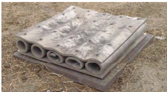
Fig. 5. Deformed elements as a result of the explosion
