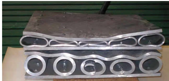
Fig. 5. Deformed elements as a result of the explosion
