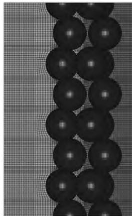
Fig. 6. FE model representing iron particles chain
