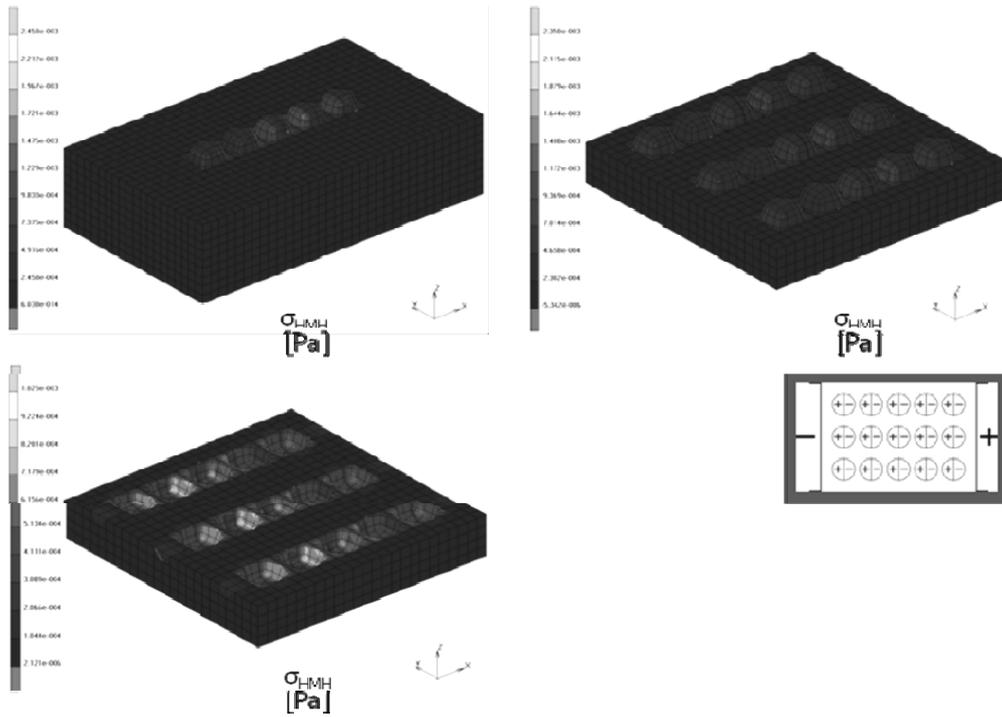
Fig. 5. Results of MRE microstructure numerical model analysis for magnetic load consideration
