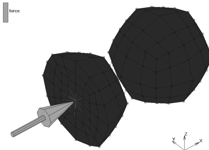
Fig. 4. Applied force simulating magnetic field influence
