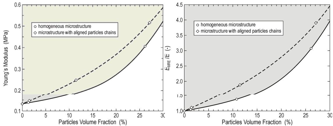
Fig. 8. Influence of the iron volume fraction on the Young's modulus of the magnetorheological elastomer (a) ; Increase of the Young's modulus value in comparison with a pure elastomer (b)
