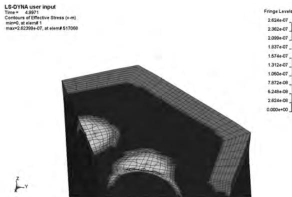
Fig. 7. Results of MRE microstructure numerical model analysis for magnetic load consideration
