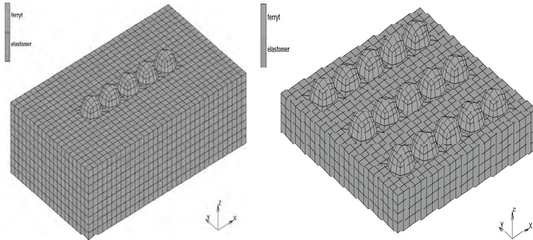
Fig. 3. Numerical model of MRE microstructure made of solid elements
