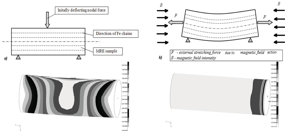
Fig. 9. Stages of MRE numerical analysis: initial bending (a), magnetic field influence consideration (b) and respective deformation fringes above
