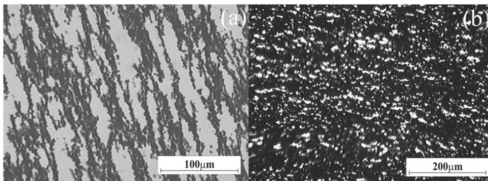
Fig. 2. Microstructure of PU cured under magnetic field of 300 mT, filled with carbonyl-iron particles: (a) 11.5 vol. %, (b) 33 vol. % [8]
