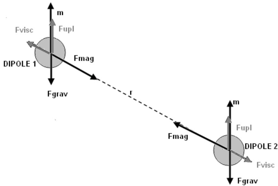
Fig. 2. Forces appeared in system of two dipoles interacting in magnetic field
