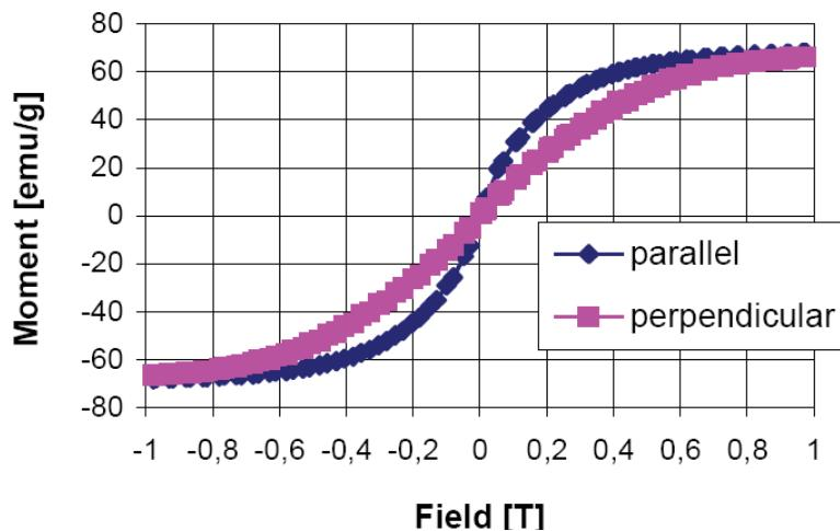
Fig. 3. Magnetic properties of MREs with 11.5 vol.% Fe, cured under magnetic field strength of 0.3 T [8]
