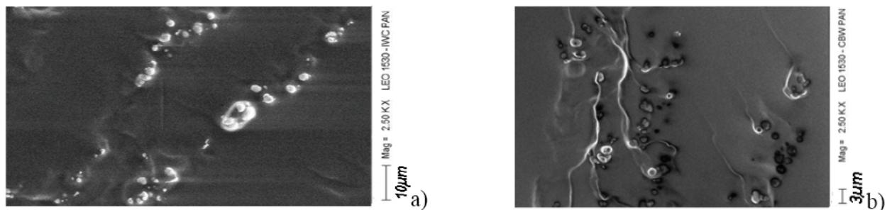
Fig. 1. SEM images of MRE obtained from PU 80/20 filled with 11.5 vol. % of carbonyl-iron particles, cured under magnetic field of a) 100 mT, b) 300 mT [6]
