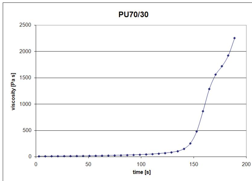
Fig. 4. Time dependence of elastomer viscosity during cross-linking
