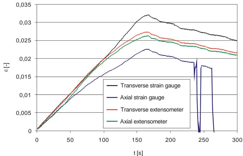
*Fig. 5. Strains versus time recorded by strain gauges and extensometers for the selected specimen*
