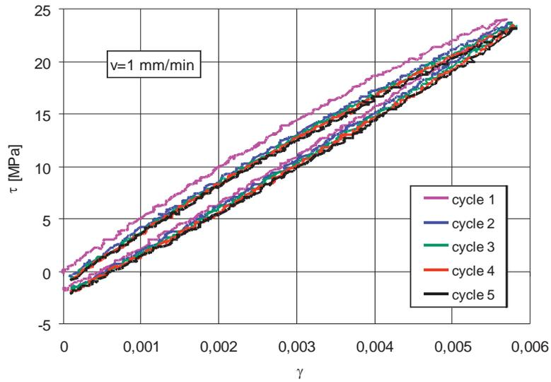
Fig. 7. The  $\tau$ - $\gamma$  diagram for  $v = 1$  mm/min (specimen No. 8)
