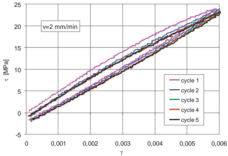
Fig. 8. The  $\tau$ - $\gamma$  diagram for  $v = 2$  mm/min (specimen No. 9)
