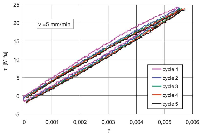
Fig. 9. The  $\tau$ - $\gamma$  diagram for  $v = 5$  mm/min (specimen No. 10)
