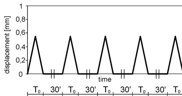
*Fig. 6. The loading program for testing selected factors in the shear test*
