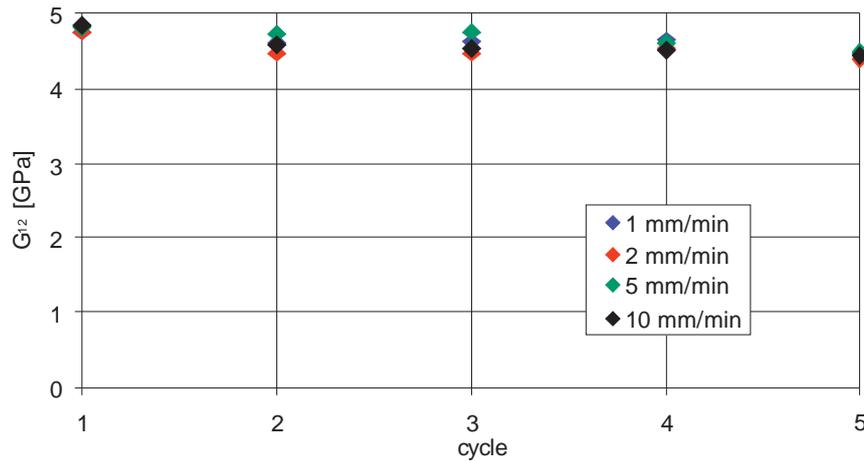
Fig. 14. The dependence of the shear modulus on a number of the loading cycles and on the crosshead rate
