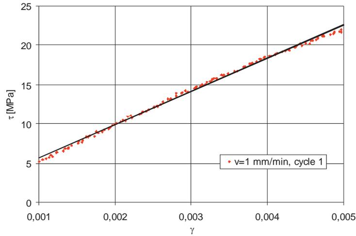
Fig. 12. The  $\tau$ - $\gamma$  diagram for  $v = 1$  mm/min in a cycle load its linear regression for  $\gamma = 0.0010 \div 0.0050$  (specimen 8)
