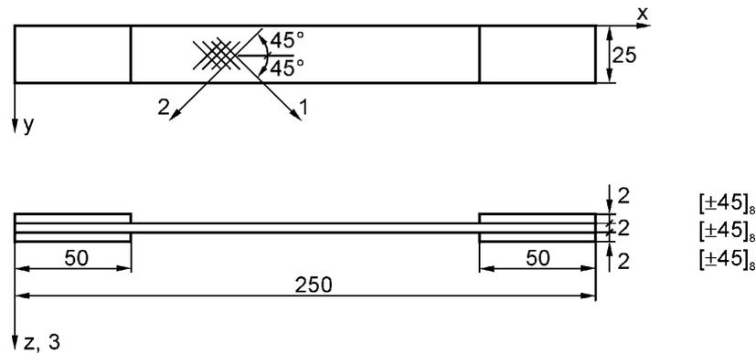
Fig. 1. A shape and geometry of the specimen, according to Ref [1]
