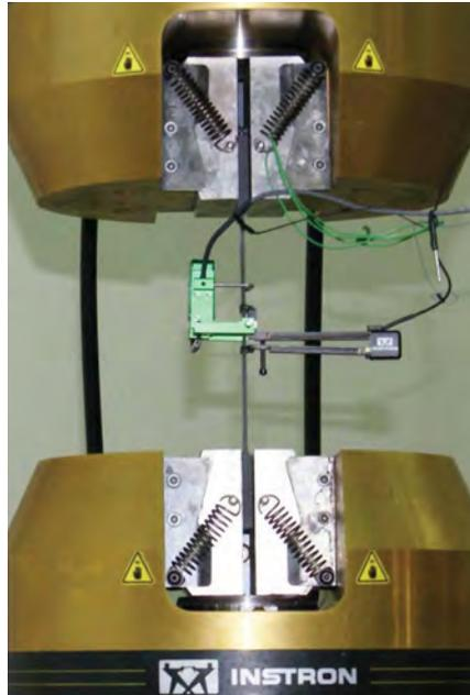
*Fig. 3. View of a specimen mounted in the hydraulic wedge grips*
