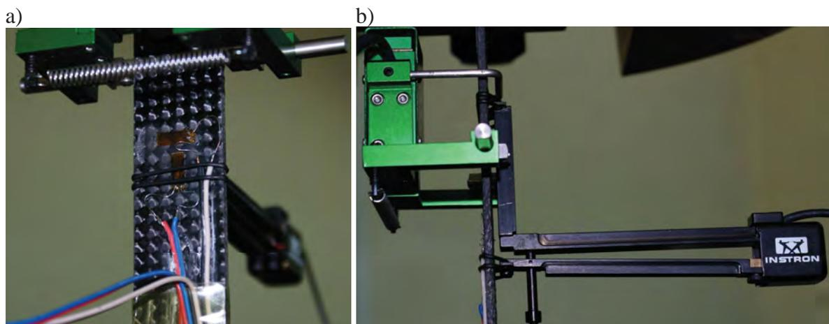
*Fig. 4. A specimen with installed sensors: a) strain gauges b) extensometers*
