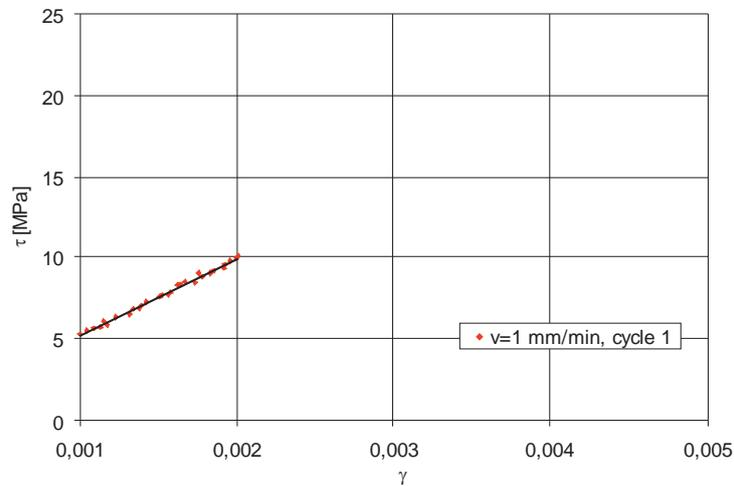
Fig. 13. The  $\tau$ - $\gamma$  diagram for  $v = 1$  mm/min in a cycle load its linear regression for  $\gamma = 0.0010 \div 0.0020$  (specimen 8)
