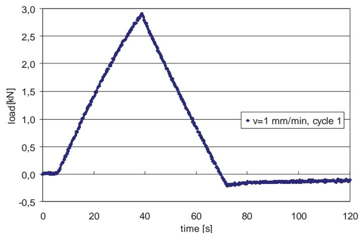
Fig. 11. The axial tensioning force versus time for  $v = 1$  mm/min in cycle 1 (specimen No. 8)
