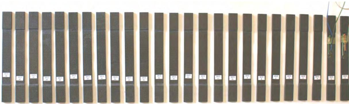
Fig. 2. Specimens for the shear test
