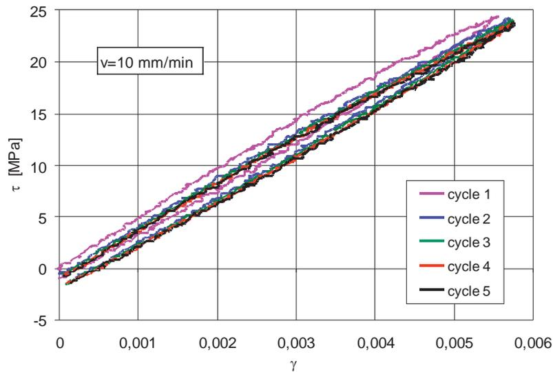
Fig. 10. The  $\tau$ - $\gamma$  diagram for  $v = 10$  mm/min (specimen No. 11)
