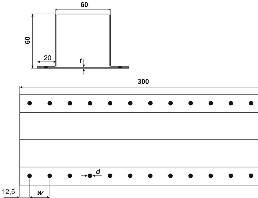
Fig. 1. The base dimensions of the top-hat profile cross sections:  $t$  - thickness,  $w$  - spot weld pitch distance,  $d$  - spot weld diameter
