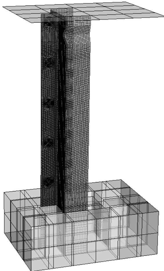
*Fig. 3. Discrete model of the crushed specimen and clamping base*
