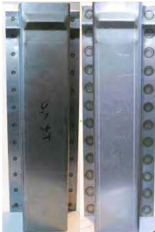
Fig. 2. Top-hat thin-walled beams triggered before crushing (profiles with two size of spot welds  $d = 4\text{mm}$  and  $d = 8\text{mm}$ )
