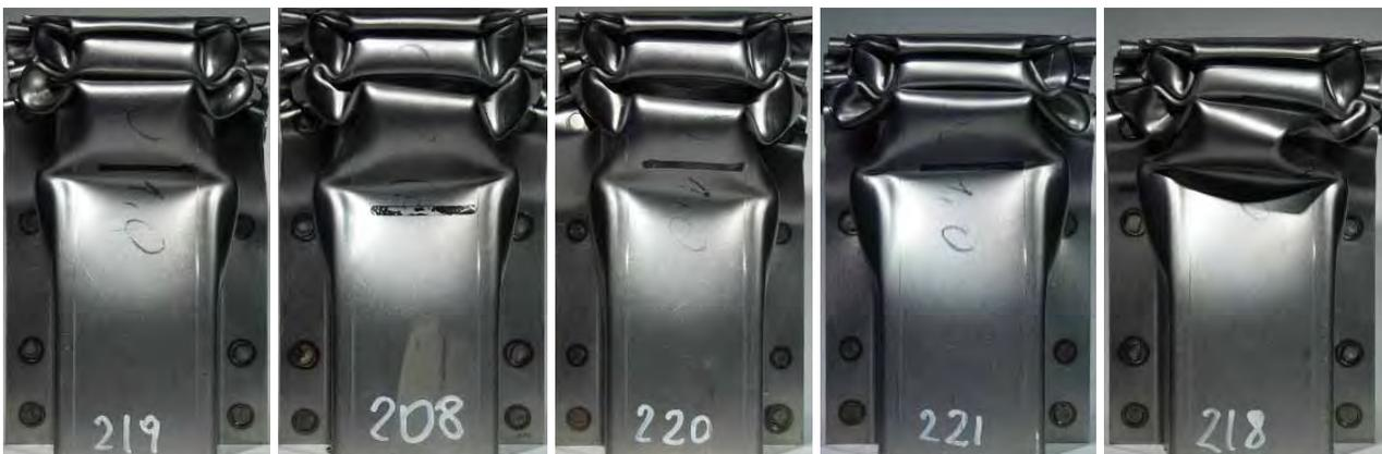
Fig. 6. Specimens TH\_DP800\_100\_50x8 – final deformation (front view)
