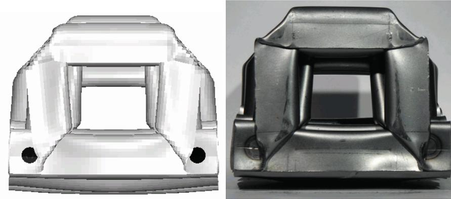
Fig. 4. Specimen TH\_DP800\_100\_50x8 – final deformation (top view)
