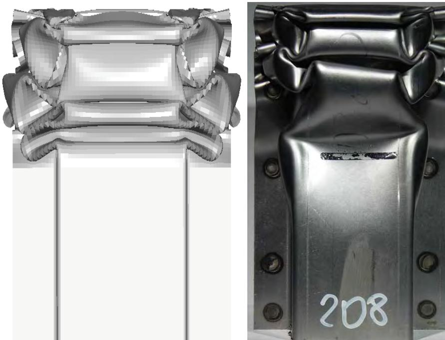
Fig. 5. Specimen TH\_DP800\_100\_50x8 – final deformation (front view)
