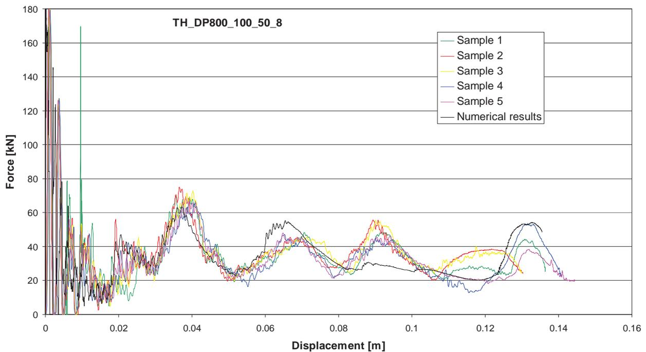
Fig. 7. Force-displacement (shortening) characteristic – top-hat specimens
