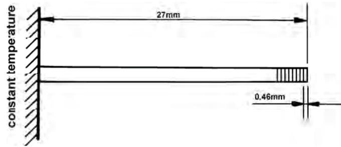
Fig. 6. Mullite rod considered as a one-dimensional system subdivided for numerical solution. Rod is 27 mm long. Calculations were performed for a 46 mm rod. Calculations showed that heat pulse applied at right end did not penetrate 27 mm in 20 second-the test time
