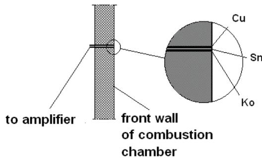
Fig. 12. Schematic view of thermocouple joint in the front wall of the combustion chamber; Cu-copper wire, Ko-constantan wire, Sn-tin thin layer as indirect metal
