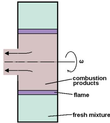
Fig. 9. Side view of flame propagating in a rotating cylindrical combustion chamber shown in a form of schematic diagram
