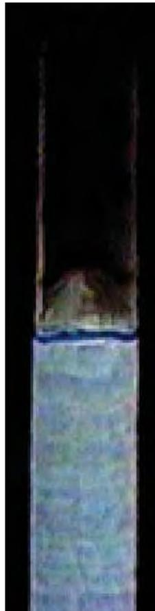
Fig. 1. Schlieren picture of flame propagating downward in a lean limit mixture (6%CH<sub>4</sub>). Dark patch seen at the top part of the tube is made by condensation of water vapour
