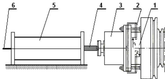
Fig. 11. Schematic diagram of the experimental apparatus for measuring wall temperature: 1-combustion chamber, 2-thermoelectric sensor, 3-system of amplifiers, 4-flexible clutch, 5-mercury commutator, 6-signal wires
