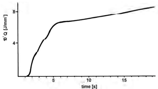
Fig. 7. Calculated heat transfer to the gauge from lean limit downward propagating flame (6%CH<sub>4</sub>)
