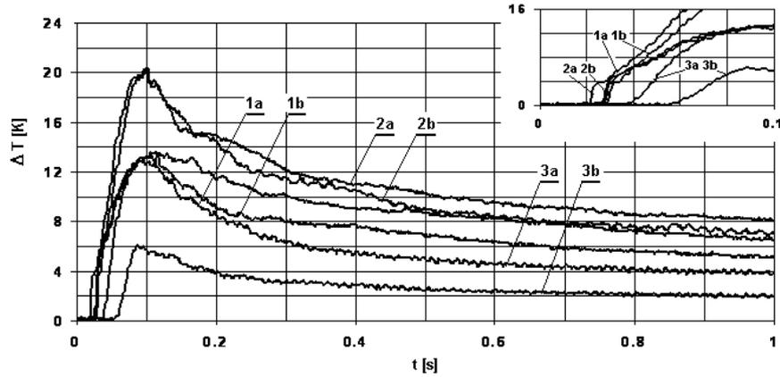
Fig. 13. Measured profiles of temperature changes in the combustion chamber wall surface. Methane/air mixture 8.45%CH<sub>4</sub>; 1a, 1b - T<sub>1</sub>, T<sub>2</sub>, rotational speed 1000rpm, 2a, 2b, - T<sub>1</sub>, T<sub>2</sub>, rotational speed 3000rpm, 3a, 3b, - T<sub>1</sub>, T<sub>2</sub>, rotational speed 5000rpm (in right top edge of the figure initial part of temperature rise is shown in detail)
