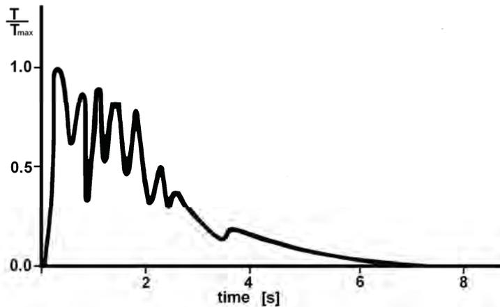
Fig. 2. Typical record of temperature measured behind flame front shown in Fig. 1
