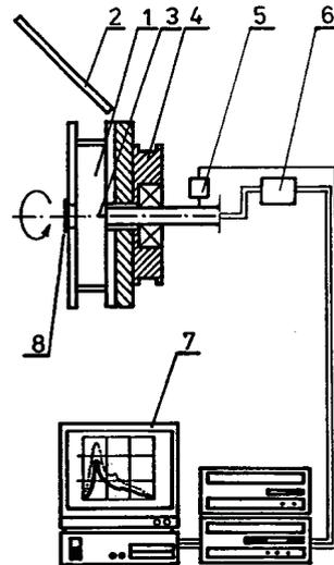
Fig. 10. Experimental set-up: 1-cylindrical chamber (with venting orifice in axis of rotation), 2-mirror, 3-ignitor, 4-V-belt wheel, 5-solenoid valve, 6-mixture supply, 7-PC, 8-tissue paper on the outflow orifice
