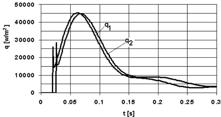
Fig. 14. Calculated heat flux density at the wall for methane/air mixture 8.45%CH<sub>4</sub> and rotational speed 3000 rpm: Heat  $q_1$  is for a radius  $r_1=23$  mm and  $q_2$  for  $r_2=28$  mm
