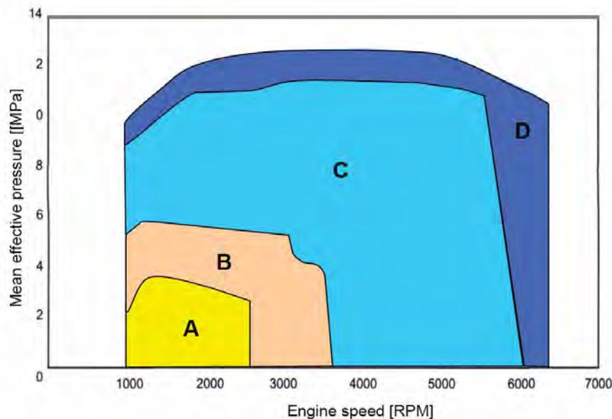
Fig. 2. General characteristics of combustible mixture composition of an engine burning of lean layered mixtures
