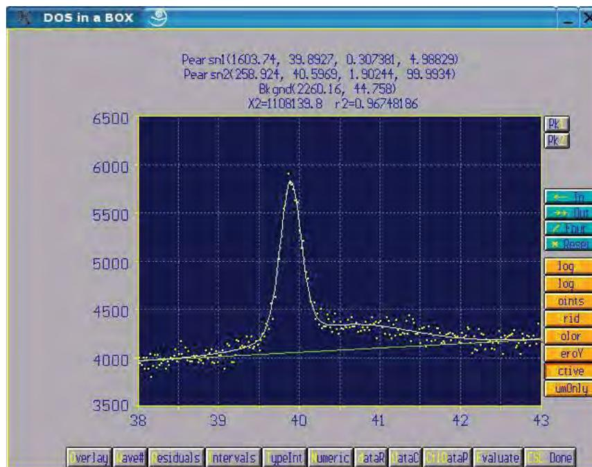
Fig. 5. Fragment of diffraction spectrum of Pt/Rh-MgO/CeO<sub>2</sub>/Al<sub>2</sub>O<sub>3</sub> reactor surface
