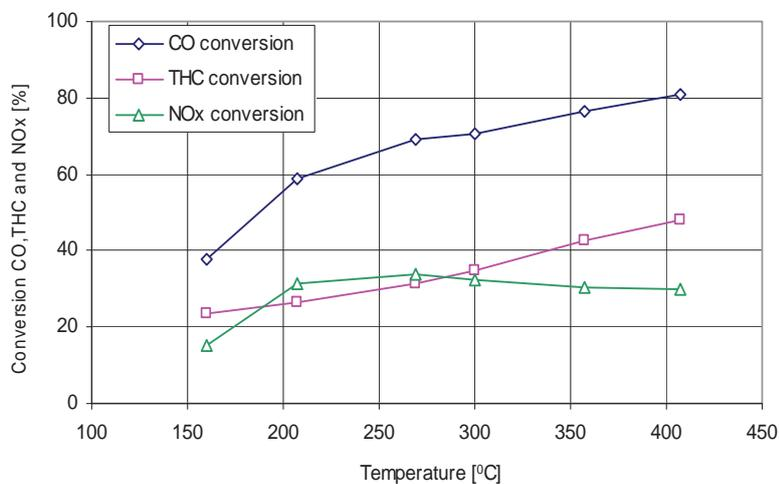
Fig. 12. CO, THC and NOx as function of catalytic process temperature during combustion of stoichiometric mixture
