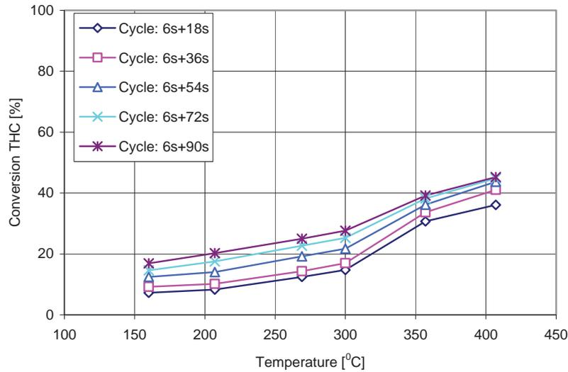
Fig. 9. Calculation results of THC conversion as function of catalytic process temperature for assumed cycles (reduction period + storage period)
