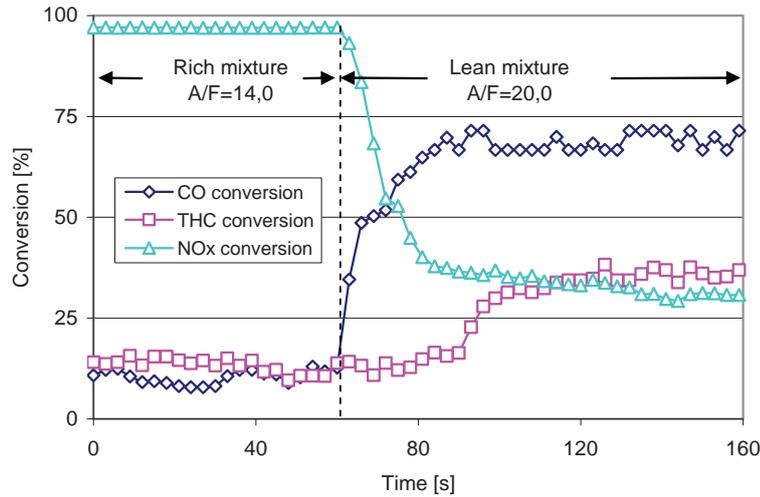
Fig. 7. Examples of calculation results of CO, THC and NOx conversion at 269°C during 60 seconds engine run on rich mixture, and 100 seconds on lean mixture
