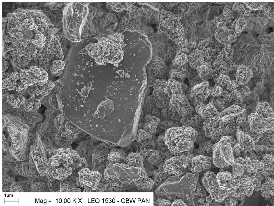
Fig. 4. Active surface of Pt/Rh-MgO/CeO<sub>2</sub>/Al<sub>2</sub>O<sub>3</sub> reactor, magnification 10 000×, scanning electron microscope (SEM)
