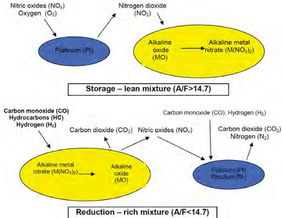
Fig. 3. Reaction diagram of storage and reduction of nitric oxides in catalytic reactor containing oxides of alkaline metals and of rare earths metals
