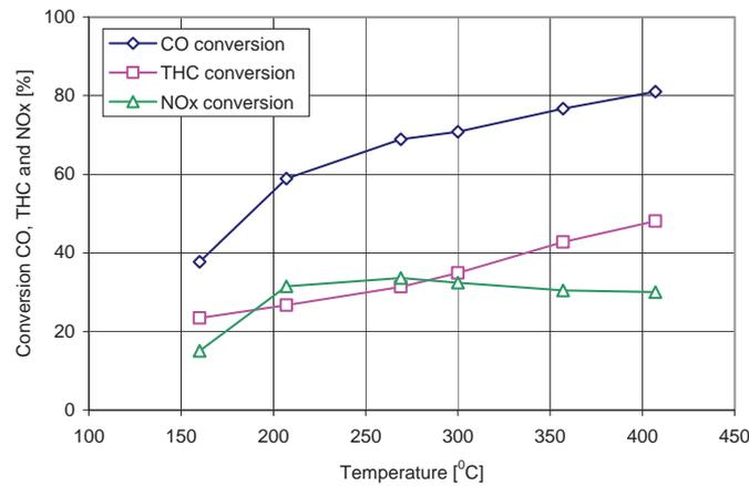
Fig. 11. CO, THC and NOx conversion during combustion of lean mixture A/F=20.0 as function of temperature
