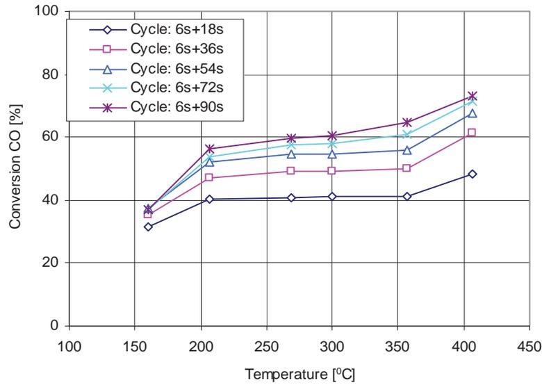
Fig. 8. Calculation results of CO conversion as function of catalytic process temperature for assumed cycles (reduction period + storage period)
