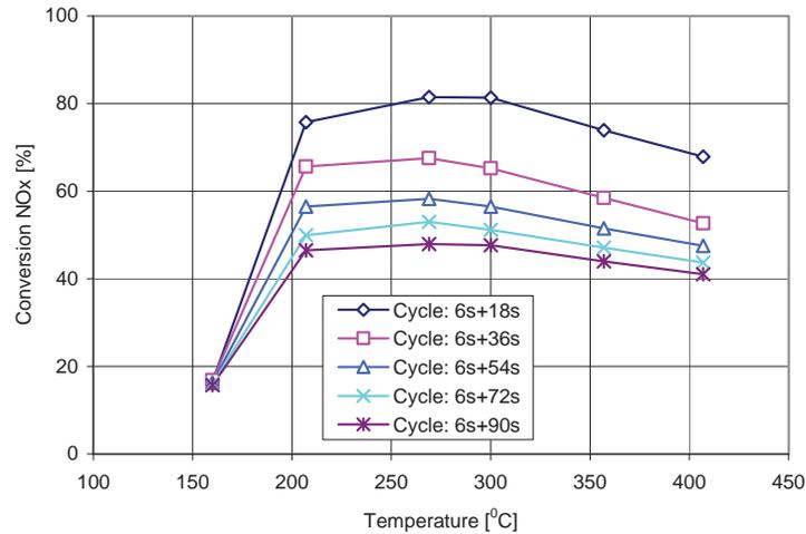
Fig. 10. Calculation results of NOx conversion as function of catalytic process temperature for assumed cycles (reduction period + storage period)
