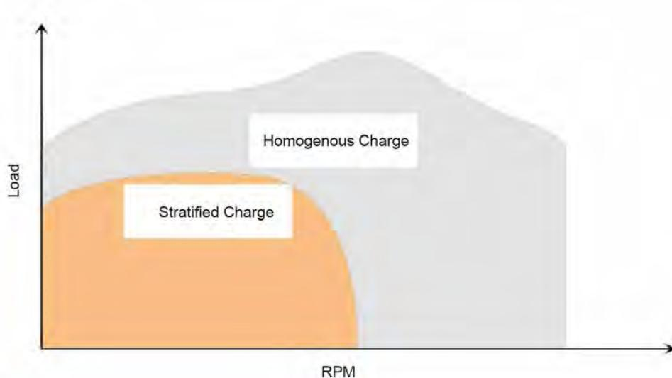
Fig. 1. Two strategies of the power supply of with the spark-ignition engines with the direct-injection: the stratified charge at small loads and rotational speeds and the homogeneous charge at big loads and rotational speeds of the engine
