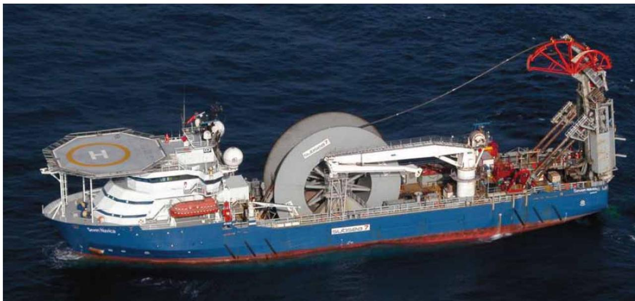
Fig. 1. Pipe laying vessel „Seven Mavica” [www.subsea7.com]
