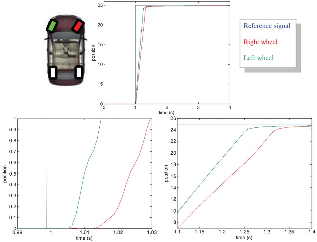
Fig. 5. Directional control action member extension pattern – the left wheel as a master, the right follows it as a slave
