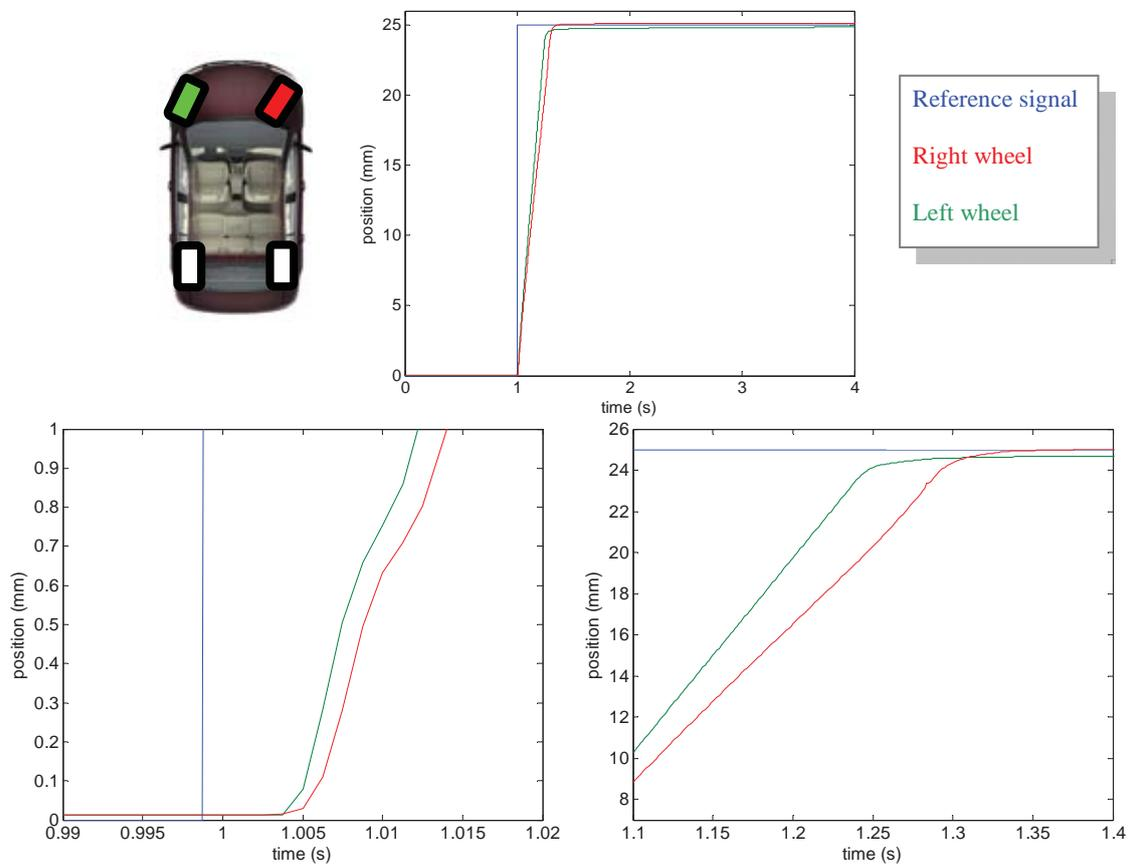
Fig. 4. Directional control action member extension pattern – each wheel controlled separately
