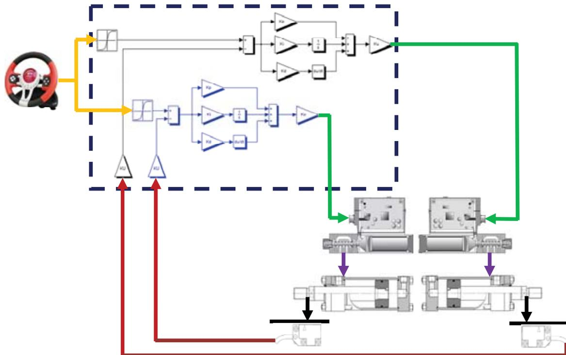
Fig. 2. Steering control layout – each wheel controlled separately
