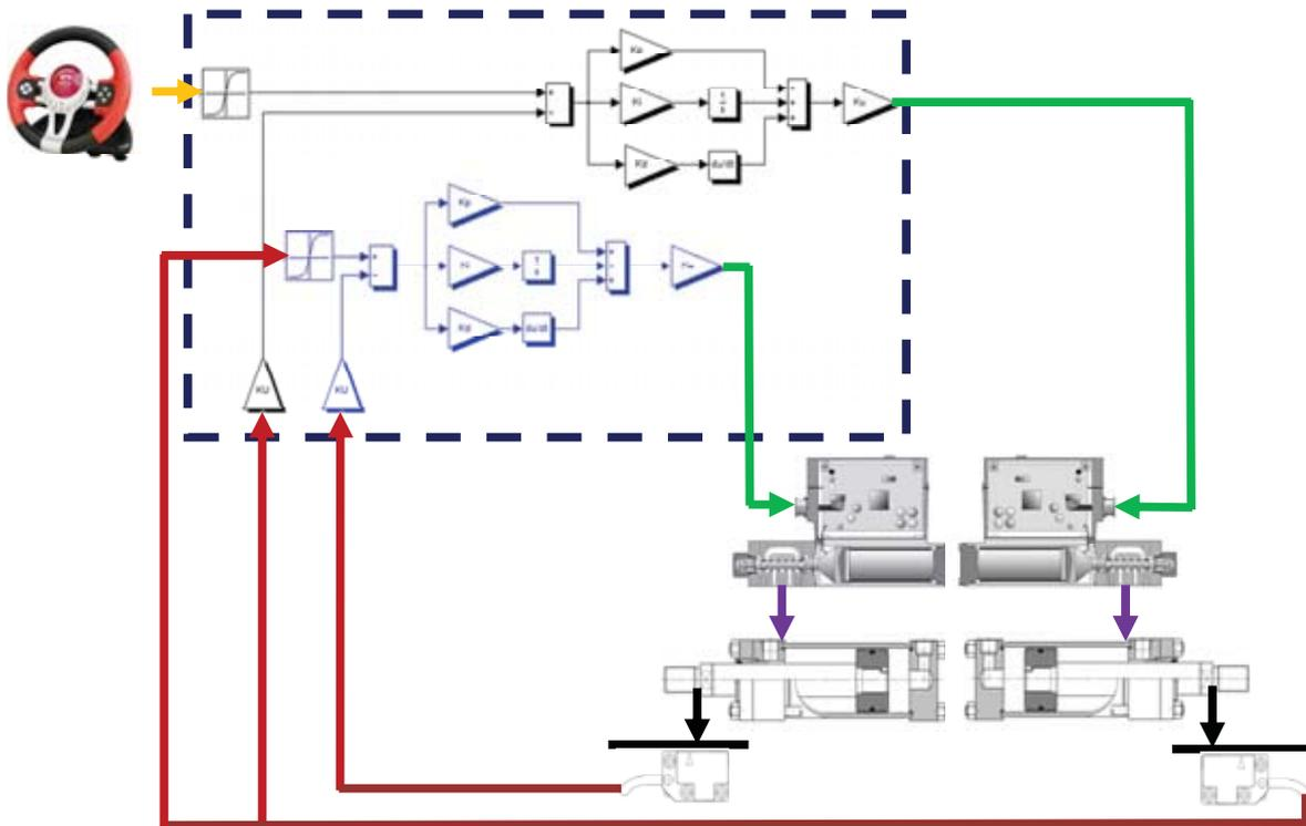
Fig. 3. Steering control layout – one wheel as a Master, the other one follows as a slave
