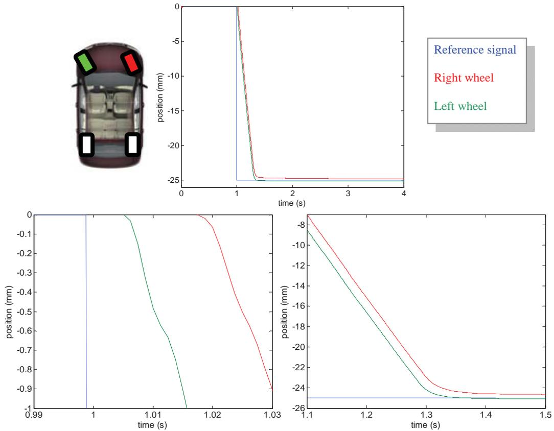
Fig. 6. The directional control action member extension pattern – the left wheel as a Master, the right one follows it as a slave
