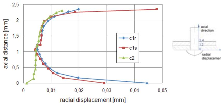
Fig. 11. Hole deformation vs. sheet axial distance
