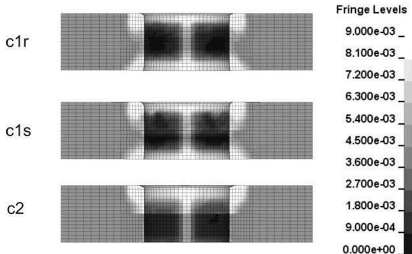
Fig. 7. Plastic strain fields in the upper and lower sheet
