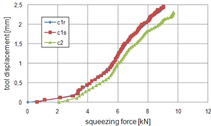
Fig. 6. Squeeze force during dynamic riveting process
