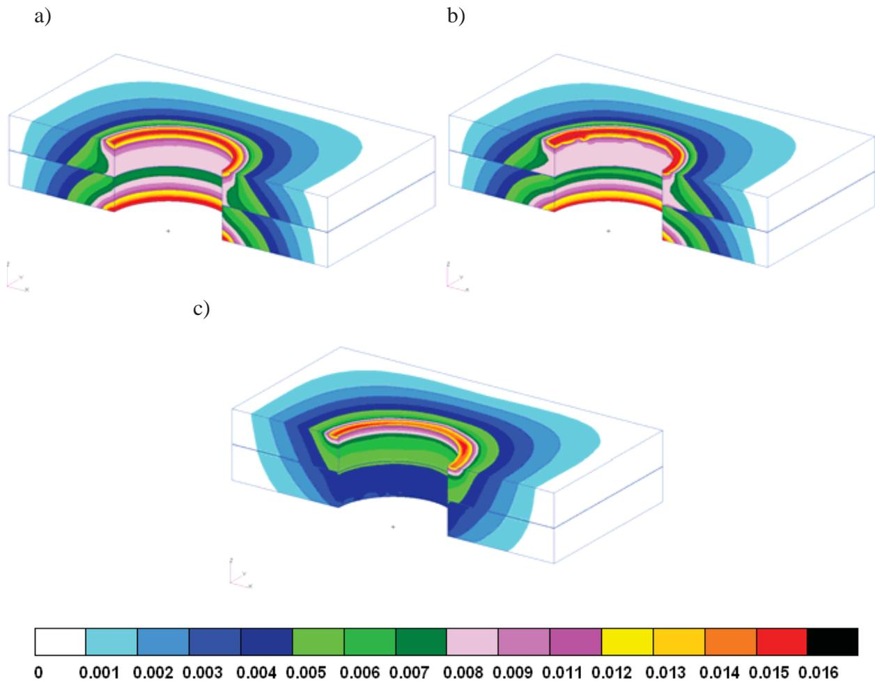
Fig. 8. Radial displacement fields in the upper and lower sheet: a) c1s; b) c1r; c) c2
