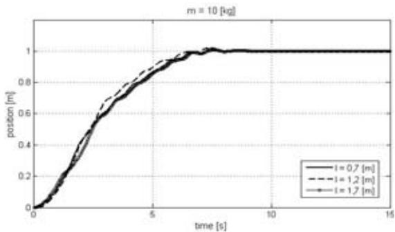
Fig. 10. Crane's position for  $m = 10$  [kg] and  $l = \{0.7, 1.2, 1.7\}$  [m]
