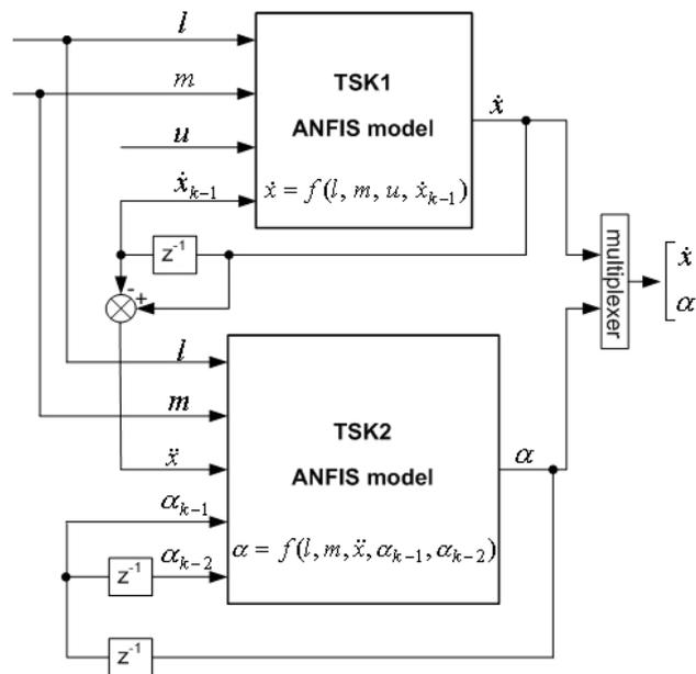
Fig. 4. ANFIS model of the crane dynamic
