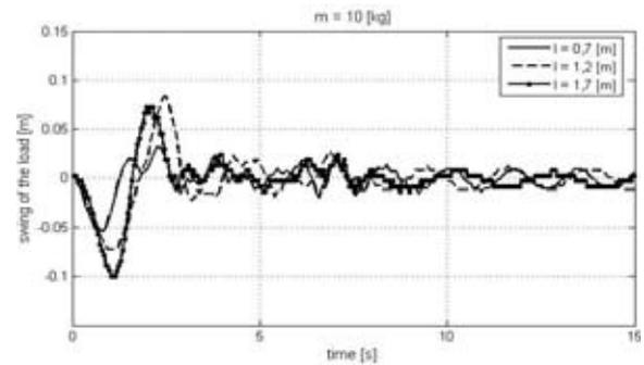
Fig. 11. Load deviation from vertical symmetry axis of the rope drum for  $m = 10$  [kg] and  $l = \{0.7, 1.2, 1.7\}$  [m]
