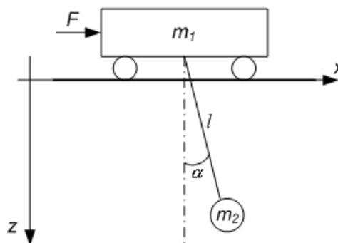
*Fig. 1. The two-mass model of a crane and shifted load*
