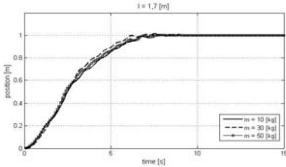
Fig. 8. Crane's position for  $l = 1.7$  [m] and  $m = \{10, 30, 50\}$  [kg]
