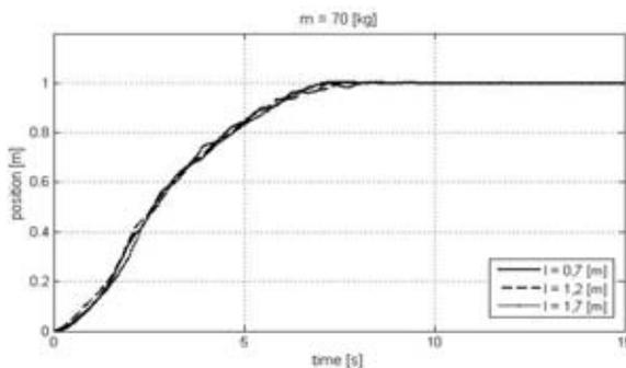
Fig. 12. Crane's position for  $m = 70$  [kg] and  $l = \{0.7, 1.2, 1.7\}$  [m]
