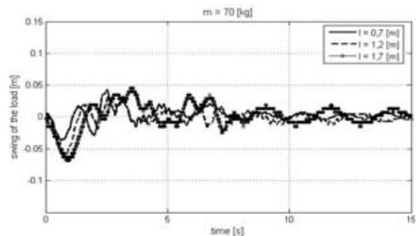
Fig. 13. Load deviation from vertical symmetry axis of the rope drum for  $m = 70$  [kg] and  $l = \{0.7, 1.2, 1.7\}$  [m]
