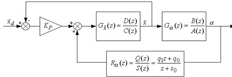
Fig. 6. Discrete anti-sway crane control system
