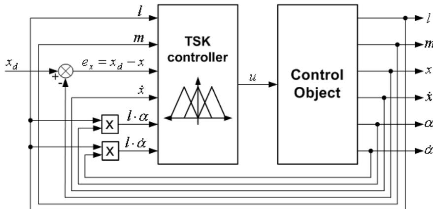
Fig. 7. Anti-sway crane control system with TSK fuzzy controller
