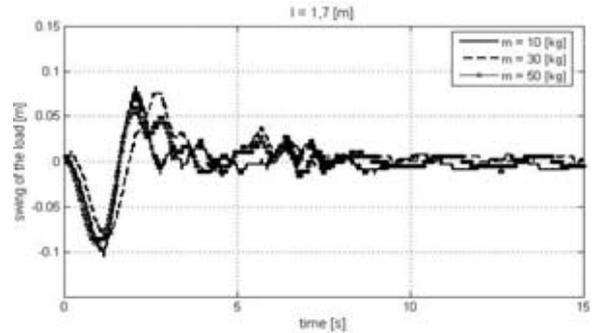
Fig. 9. Load deviation from vertical symmetry axis of the rope drum for  $l = 1.7$  [m] and  $m = \{10, 30, 50\}$  [kg]
