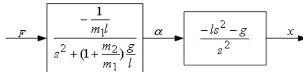
Fig. 2. Model of crane dynamic shown using continuous transfer functions
