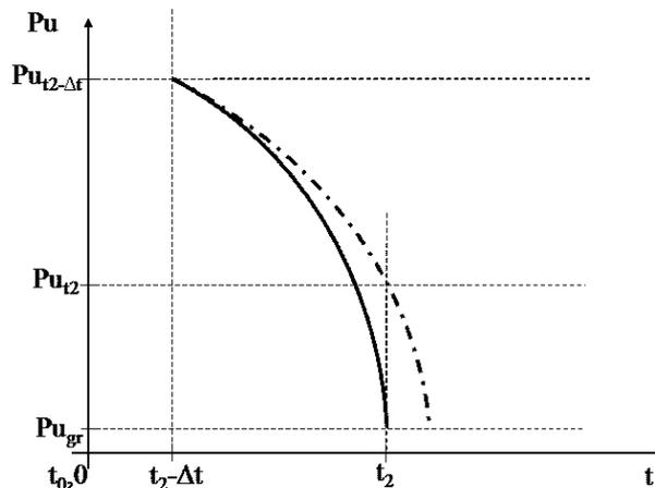
Fig. 2. The process of operational potential consumption – maintenance strategy by controlled consumption of operational potential
