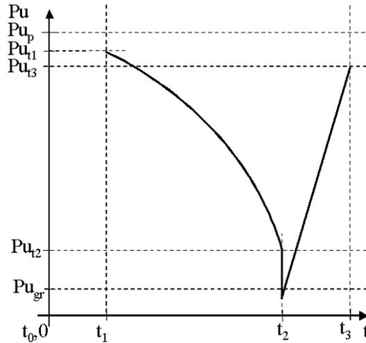
Fig. 1. The changes of operational potential amount during operating and service processes
