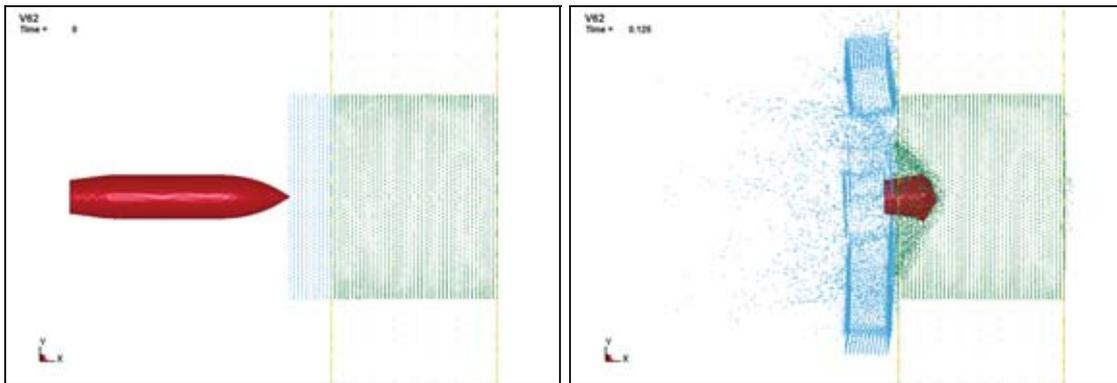
Fig. 7. Penetration of the ceramic tile/aluminium alloy plate set by 12.7 x 108 B32 hard core. Impact velocity 840 m/s, ceramic tile thickness 10 mm
