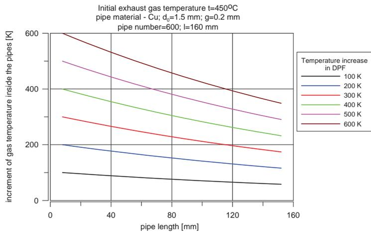
Fig. 6. Increase of the inner exhaust gas temperature along the copper pipes at different temperature increase in DPF (with initial temperature  $450^{\circ}\text{C}$ ) without radiation
