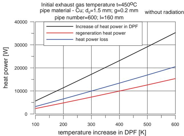
Fig. 9. Heat recovery at different increment of the temperature in DPF (without radiation)
