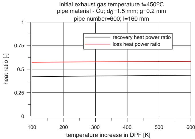
Fig. 8. Heat power of the regeneration without radiation (Cu pipes)
