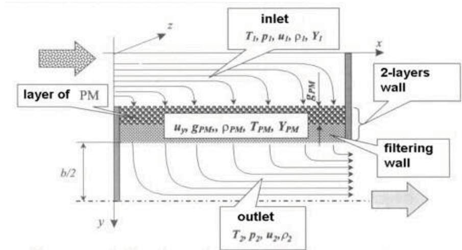
Fig. 1. One dimensional model of DPF filtration and regeneration [6]
