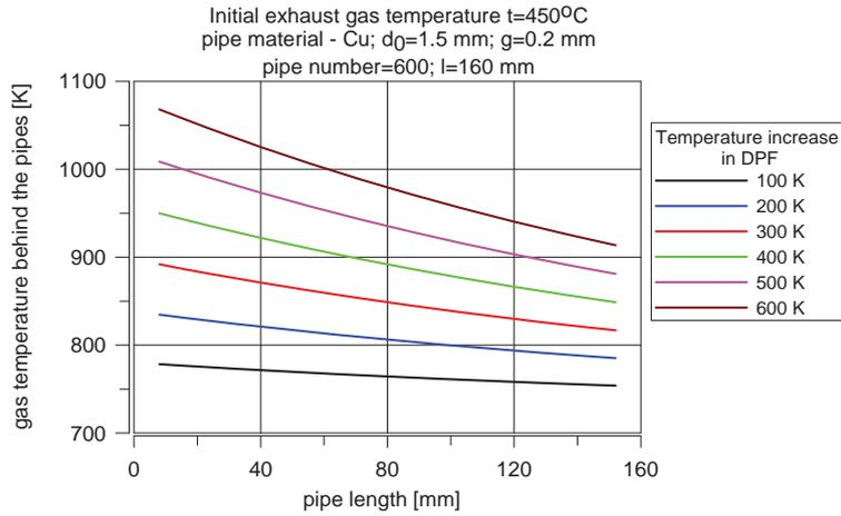
Fig. 5. Exhaust gas temperature after regeneration along the pipes at different temperature increase in DPF with initial temperature  $450^{\circ}\text{C}$  (without radiation)
