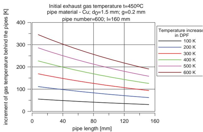
Fig. 4. Increase of the exhaust gas temperature after regeneration along the pipes at different temperature increase in DPF with initial temperature 450 °C (without radiation)
