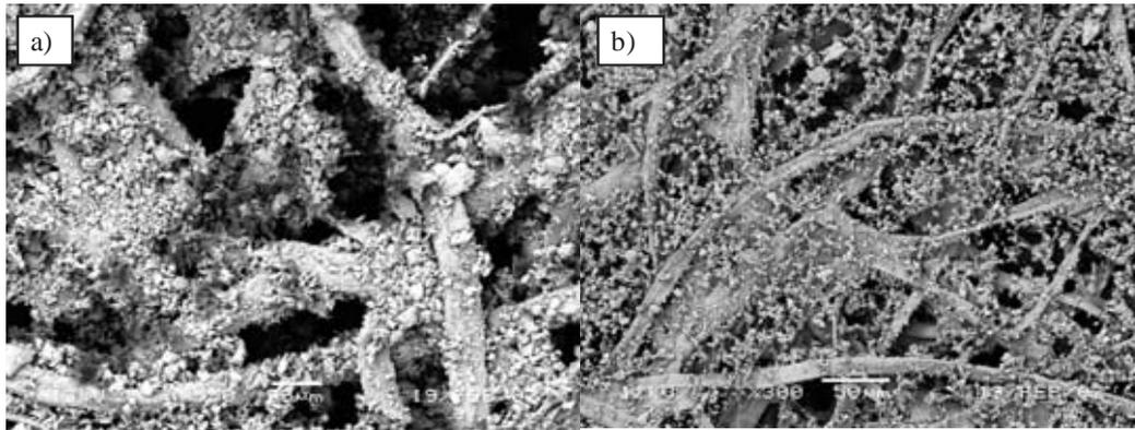
Fig. 5. Dust particle distribution on cellulose filter media – a) and on nanofiber filter media – b)
