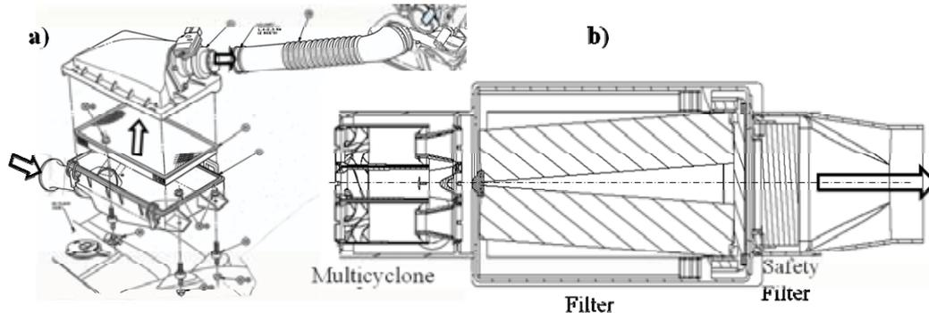
Fig. 1. Schematic view of a Panel Filter- a) Direct Flow filter- b)
