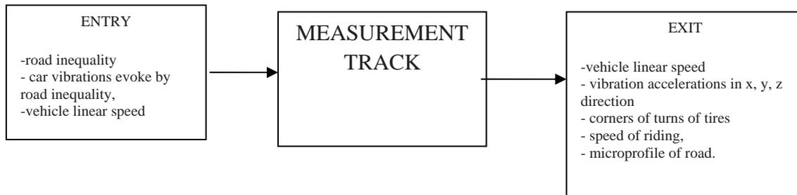
Fig. 2. Measurement track schema
