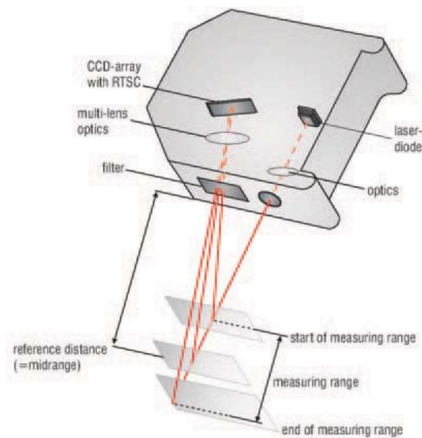
Fig. 4. Principle of the distance measurement applied in the ILD-1402 sensor
