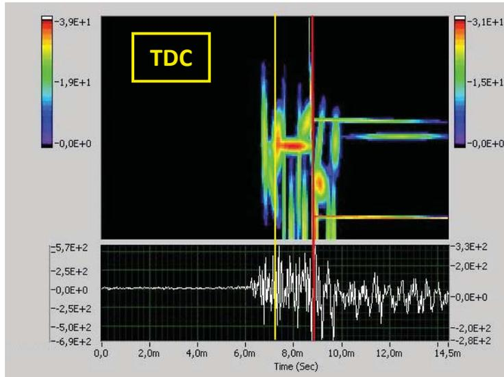
Fig. 8. Adaptive spectrogram analysis result, nominal clearance  $n = 1415 \text{ min}^{-1}$ , x-axis
