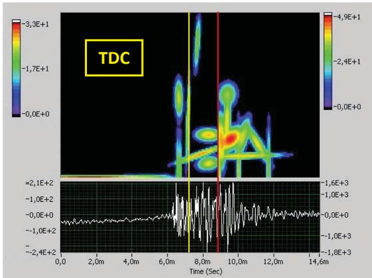
Fig. 9. Adaptive spectrogram analysis result, 2x nominal clearance  $n = 1437 \text{ min}^{-1}$ , x-axis
