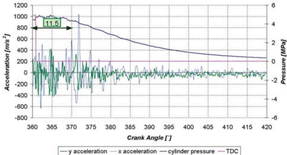
Fig. 2. Vibration acceleration amplitude angle shift for nominal clearance
