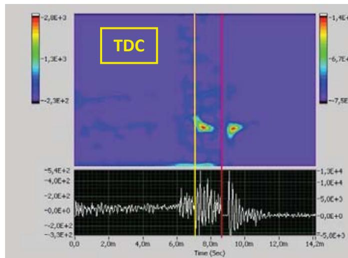
Fig. 7. Gabor analysis result, 4x nominal clearance  $n = 1415 \text{ min}^{-1}$ , x-axis
