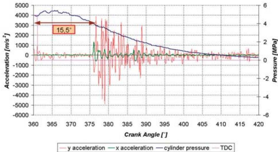
Fig. 4. Vibration acceleration amplitude angle shift for 4x nominal clearance
