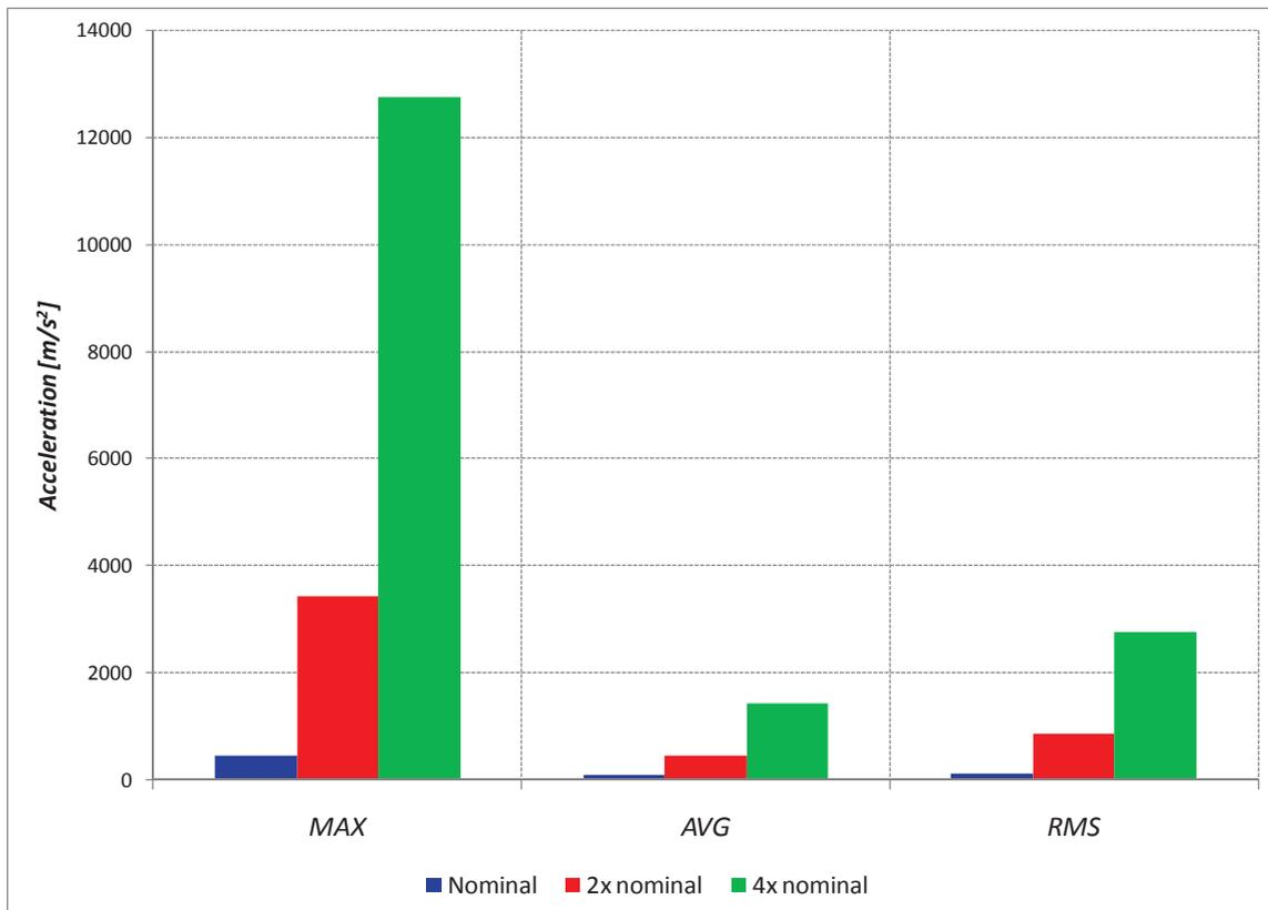
Fig. 12. Pointers calculated for acceleration signal after decomposition
