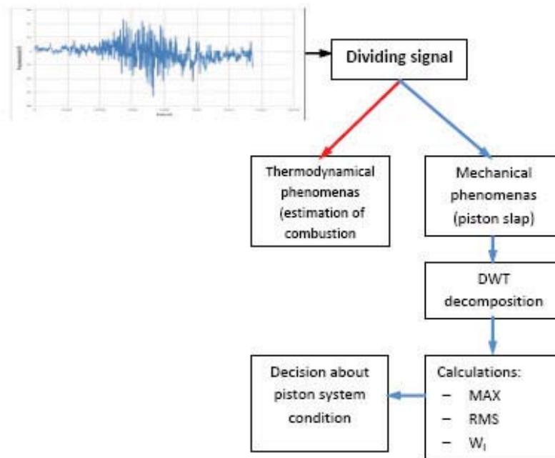
Fig. 15. Engine piston system condition algorithm
