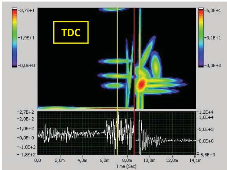
Fig. 10. Adaptive spectrogram analysis result, 4x nominal clearance  $n = 1415 \text{ min}^{-1}$ , x-axis
