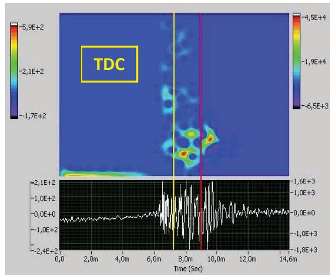
Fig. 6. Gabor analysis result, 2x nominal clearance  $n = 1437 \text{ min}^{-1}$ , x-axis
