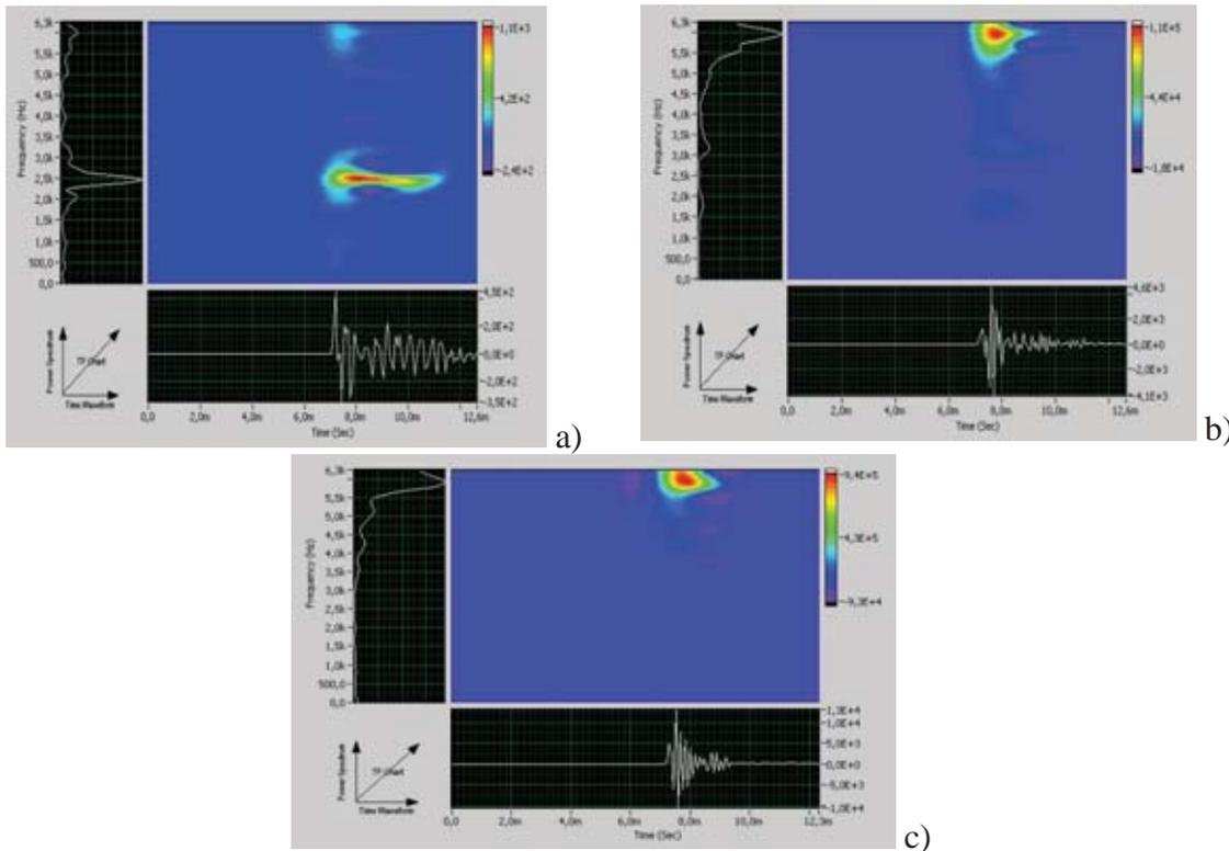
Fig. 14. Results of Gabor's analysis for signal after decomposition, a) for nominal clearance, b) for two times bigger clearance, c) for four times bigger clearance
