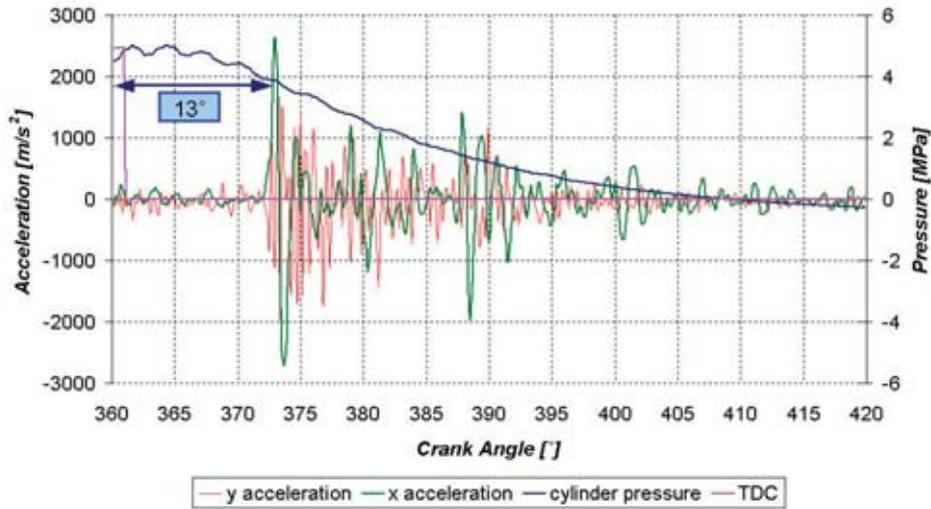
Fig. 3. Vibration acceleration amplitude angle shift for 2x nominal clearance
