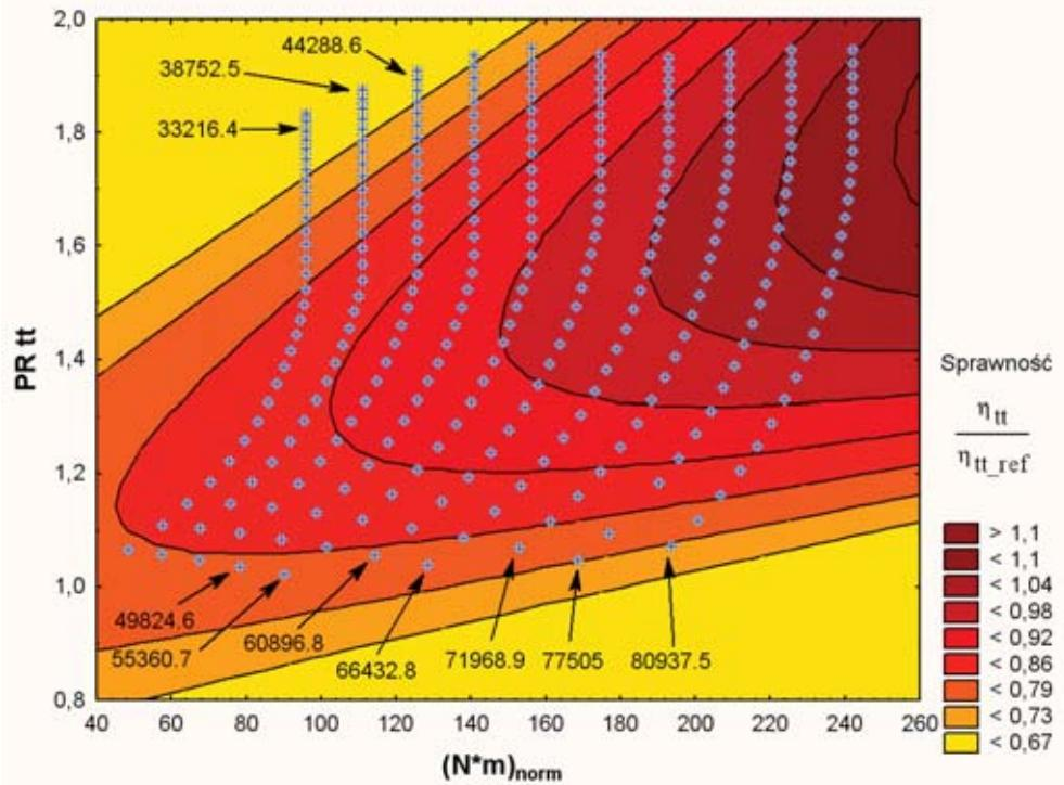
Fig. 5. Turbine to micro gasturbine performance map for different normalized rotational speed  $N_{norm} = \frac{N}{\sqrt{\frac{a_{in}}{a_{std}}}}$
