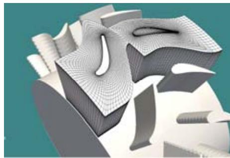
Fig. 6. Turbine geometry with O-Grid
