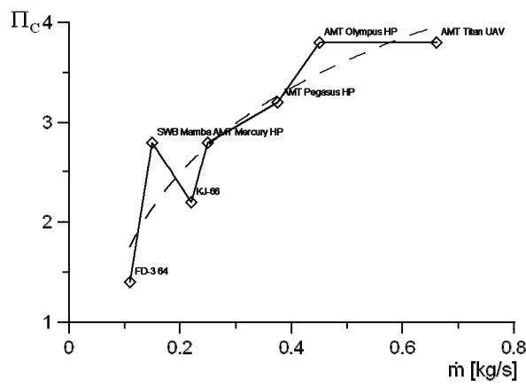
Fig. 1. Compression ratio – solution possibility
