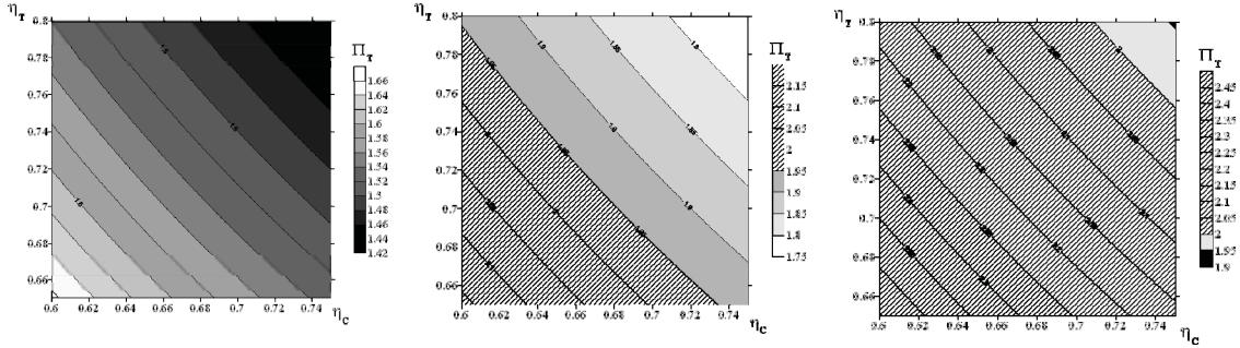
Fig. 3. Turbine expansion ratio  $\Pi_T$  as a function of compressor and turbine efficiency for mass flow rate = 0.15, 0.30 and 0.45 [kg/s]
