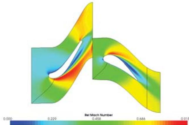
Fig. 8. Relative Mach number at middle cut of the blade
