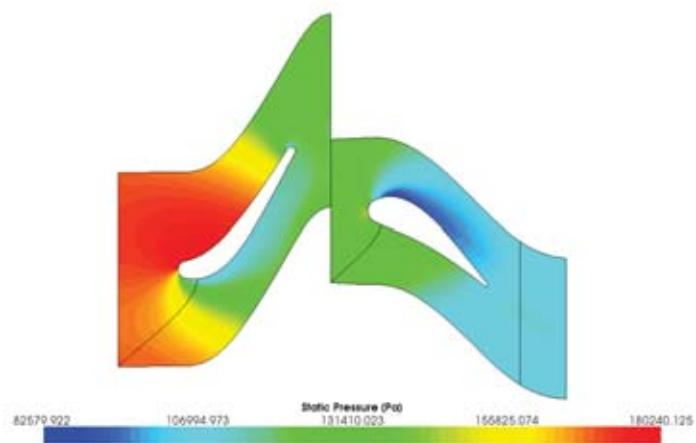
Fig. 9. Static Pressure at middle cut of the blade
