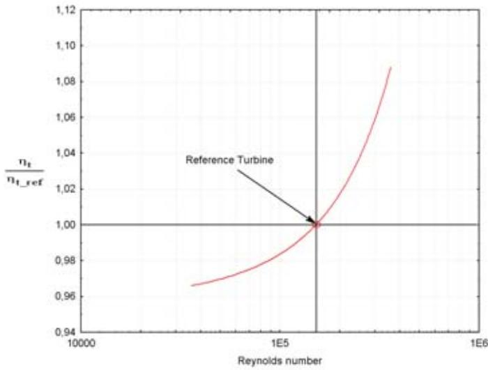
Fig. 4. Efficiency of turbine as a function of Reynolds number  $Re = \frac{\rho \cdot U \cdot D}{\mu}$  for constant specific speed coefficient
