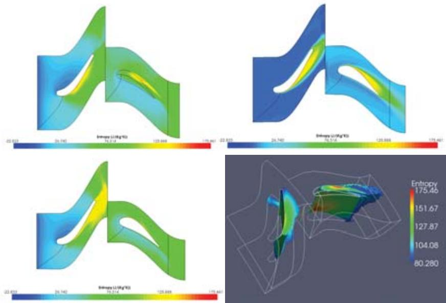
Fig. 7. 2D and 3D contours plots of Entropy (left upper corner - shroud, right upper corner - middle, left lower corner - shroud, right lower corner - 3D contours of largest entropy)
