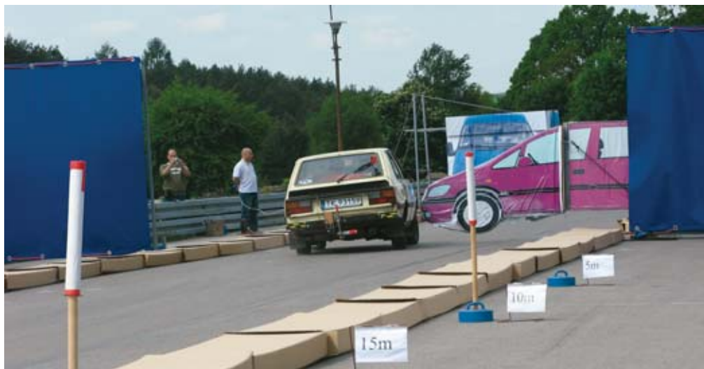
Fig. 5. Performing the manoeuvre of avoiding during tests
