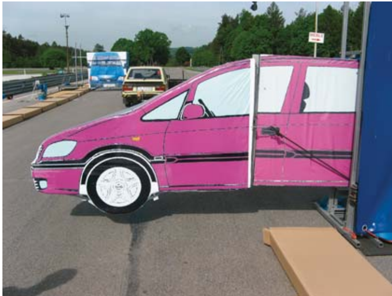
Fig. 2. An obstacle 1 mock-up made of polyurethane foam
