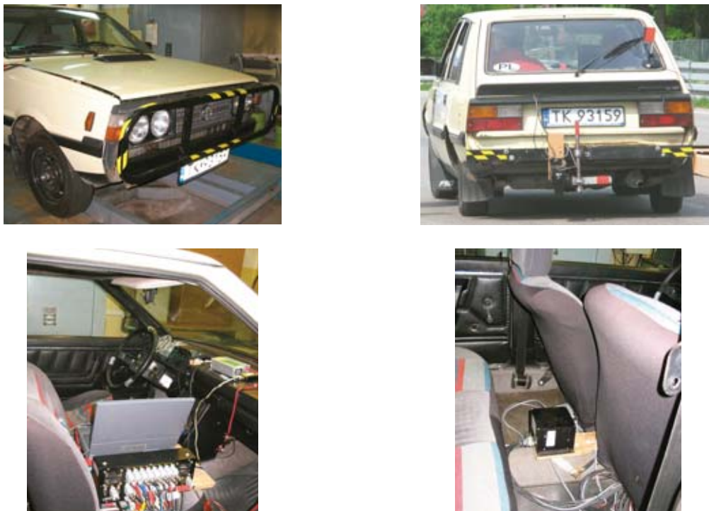
Fig. 3. The view of a testing vehicle and the part of equipment: Correvit double parameter head system (the measurement of longitudinal and lateral component of a velocity vector of a selected car point), a steering wheel angle converter with a line transmission, eight-parameter Crossbow measuring block (used for measuring yaw velocity, roll velocity, the components of longitudinal and lateral acceleration vector of a point near the mass centre). AD 12 converter with plugged cables of measured signals, controlled by a laptop computer. The car has been equipped with a special Safari type bumper protecting the car front during a collision with the obstacle
