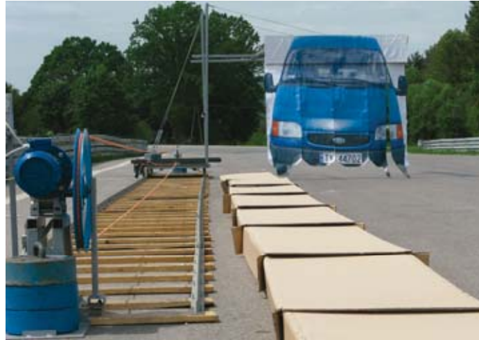
Fig. 4. The car mock-up approaching from the opposite direction – “obstacle 2”
