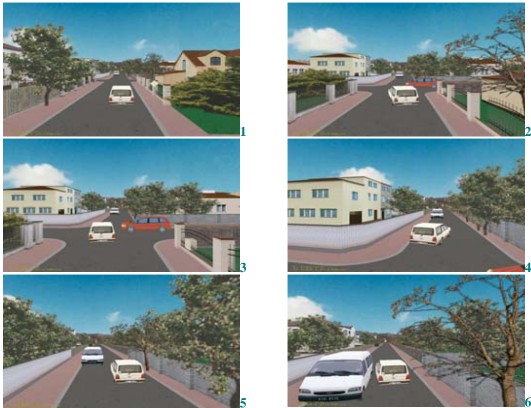
Fig. 7. Subsequent driving phases of the tested vehicle in accident situation in which the driver has avoided the accident (Driver 096, V=50\text{km/h} , S=20\text{m} , risk time 1.44s)
