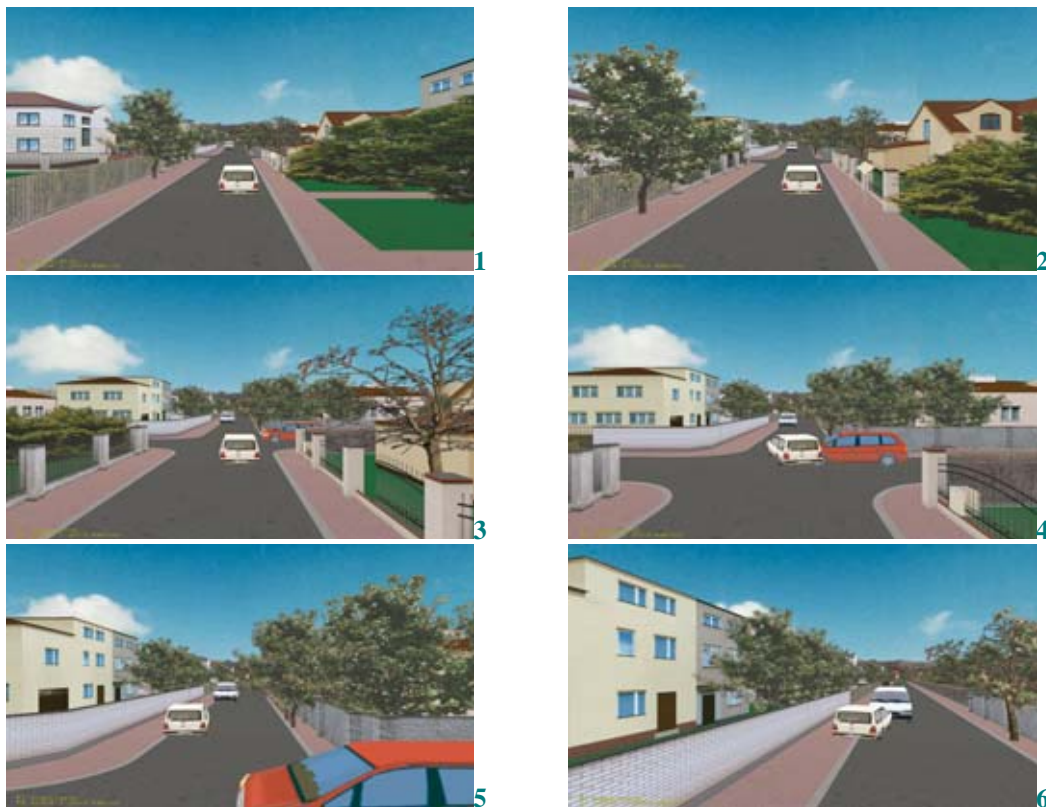
Fig. 6. Subsequent driving phases of the tested vehicle in accident situation in which the driver has failed to avoid the crash (Driver 089, V=60\text{km/h} , S=10\text{m} , risk time 0.6\text{s} )
