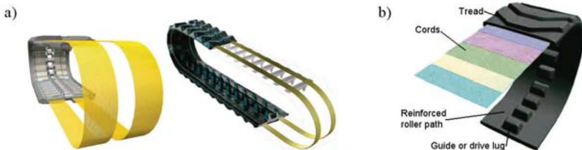
Fig. 3. Elastomer tracks for the positive (a) and friction (b) drive transmission [7]
