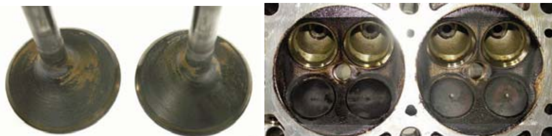
Fot. 6. Zawory dolotowe i komory spalania oceniane w procedurze CEC F-20-98 Fig. 6. Intake valves and combustion chambers evaluates according to CEC F-20-98
