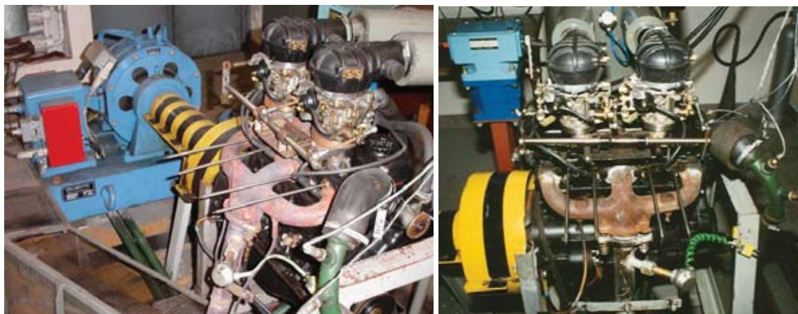
Fot. 1. Stanowisko testowe z silnikiem OPEL Kadett [ITN] Fig. 1. View of test bed with OPEL Kadett engine [ITN]
