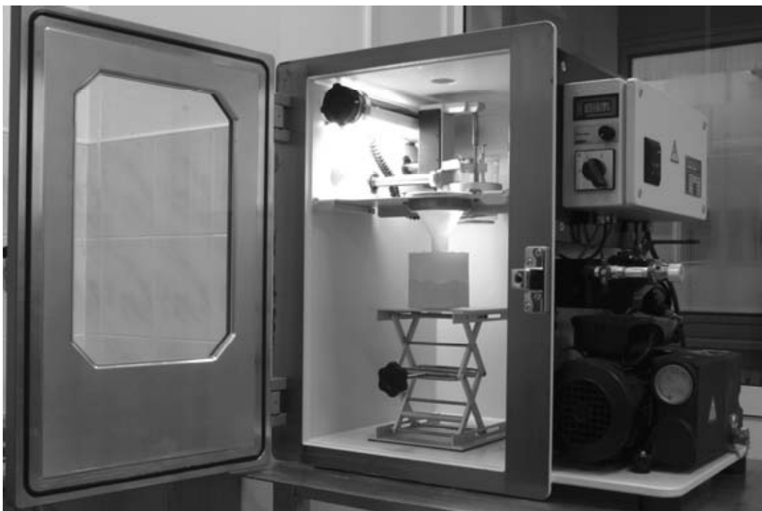
Fig. 1. Vacuum Casting apparatus, VAKUUM UHG 400 type
