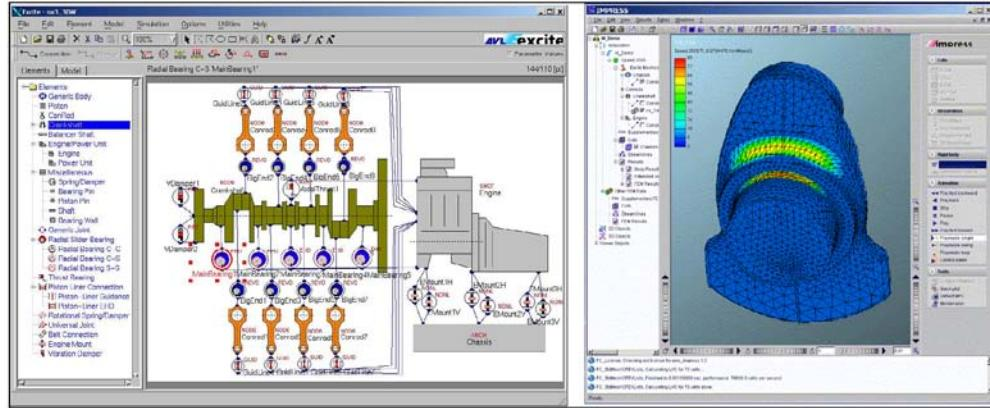
Fig. 6. System modelling and result evaluation for engine durability simulation
