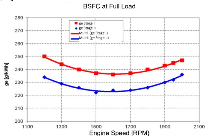
Fig. 6. Comparison of specific fuel consumption (BSFC) as an engine speed function of the tested S12-U engine with pistons made of novel composite alloy and PA alloy forged pistons at full load operation
