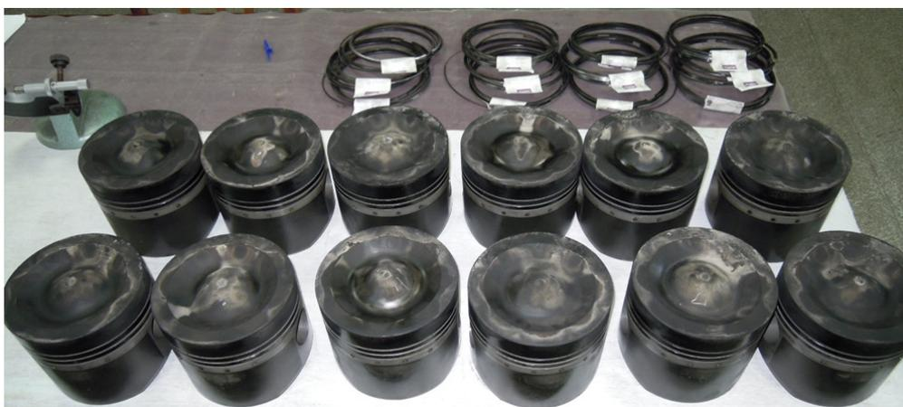
Fig. 10. View of the novel composite alloy pistons after engine testing
