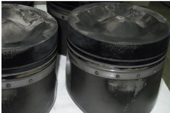
*Fig. 12. View of piston carbon deposits opposite to Fig. 11*
