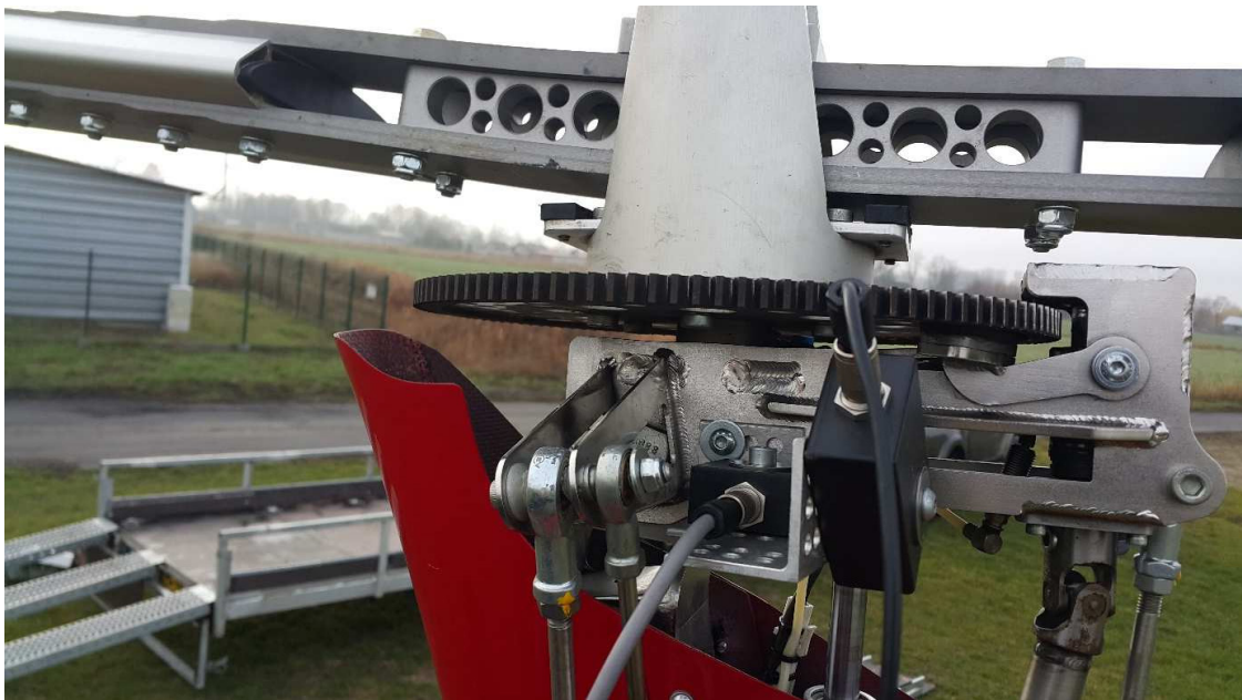
Fig. 2. Test bench – rotor head with positive coning angle hub connector and mounted sensors
