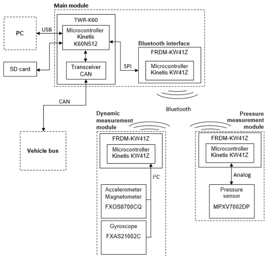
Fig. 2. The scheme of the prototype of modular monitor of car exploitation parameters in motion
