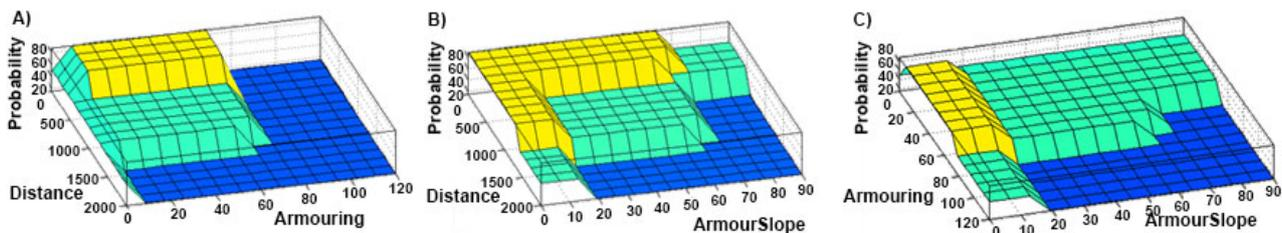
Fig. 3. Control surfaces after optimization of the system: A) Dependence of probability of armour piercing upon target distance and armour thickness, B) Dependence of probability of armour piercing upon target distance and armour slope, C) Dependence of probability of armour piercing upon armour slope and armour thickness
