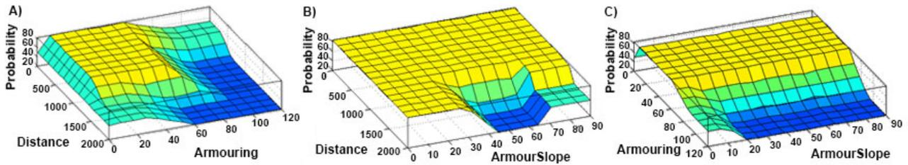
Fig. 2. Control surfaces: A) dependence of probability of armour piercing upon target distance and armour thickness, B) dependence of probability of armour piercing upon target distance and armour slope, C) dependence of probability of armour piercing upon armour slope and armour thickness
