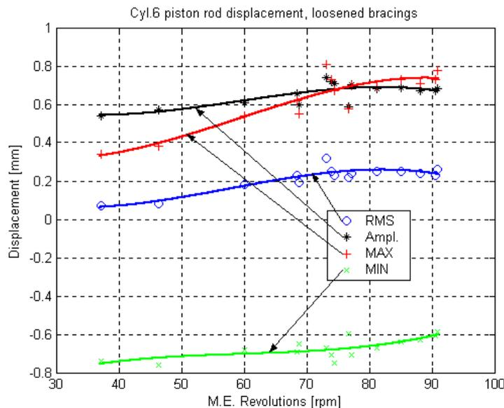
Fig. 6. The displacement of piston rod of cylinder No. 6 with loosened bracings
