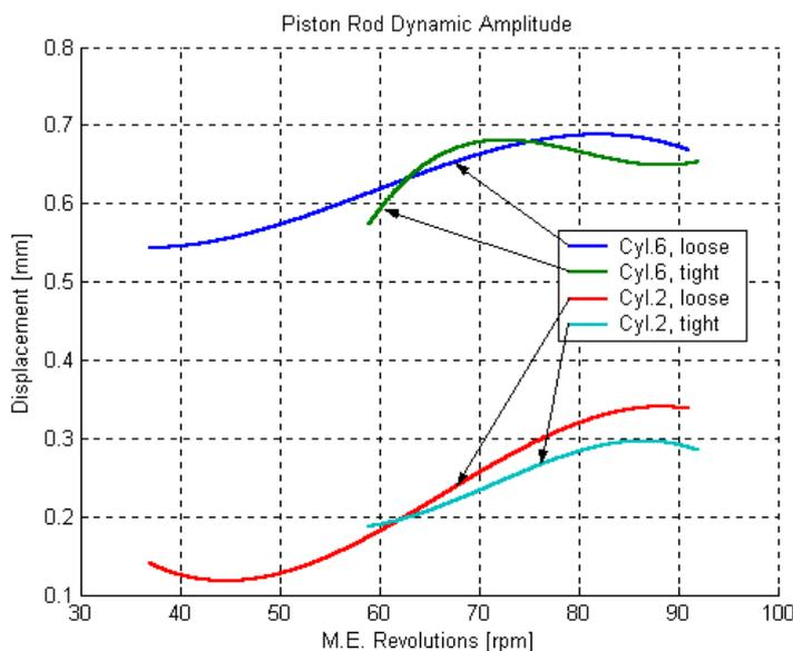
Fig. 7. The piston rod dynamic displacements
