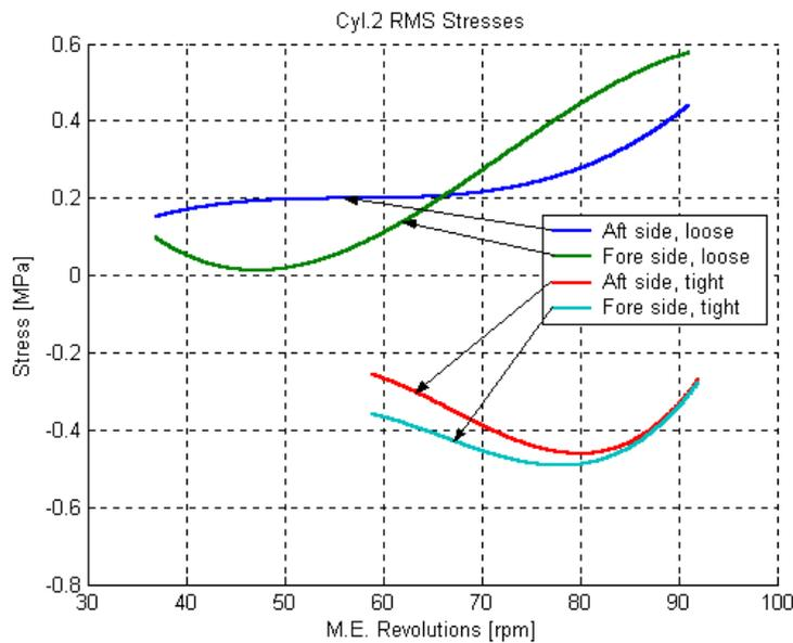
Fig. 3. RMS type stresses in the engine A-frames
