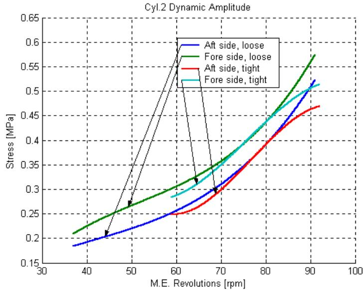
Fig. 4. Ampl. type stresses in engine A-frames
