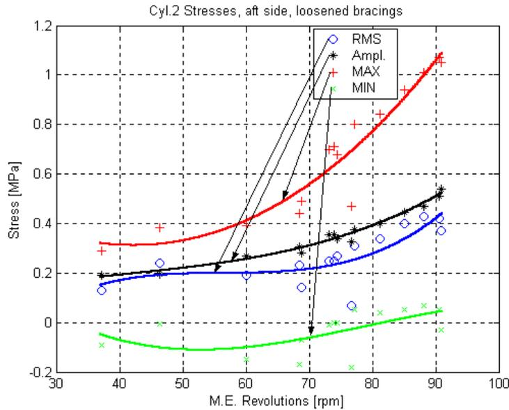
Fig. 2. Stresses in aft A-frame, in operation with loosened bracings
