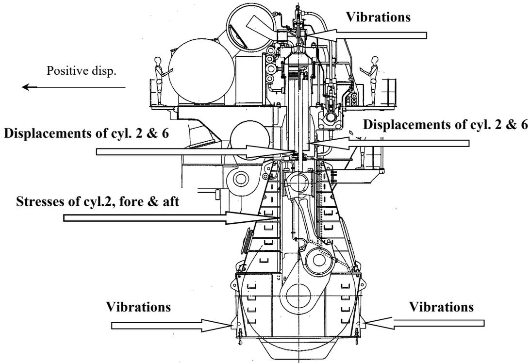
Fig. 1. An arrangement of the measuring points
