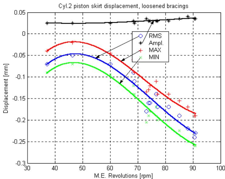
Fig. 5. The displacements of cylinder liner No. 2 (M.E. running; loosened bracings)
