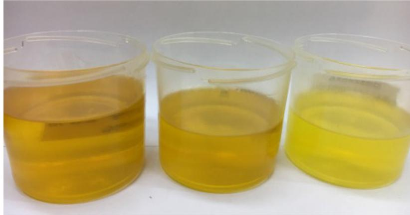
Fig. 1. Mixtures of diesel oil and methyl esters of fatty acids
