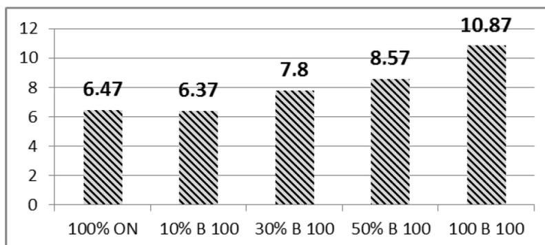
Fig. 3. Dependence of viscosity on biocomponent content
