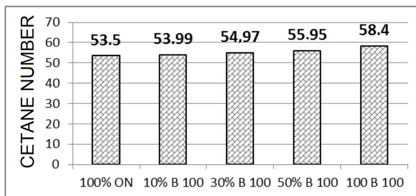
Fig. 4. Mean values of cetane number for variable contents of a biocomponent in a fuel
