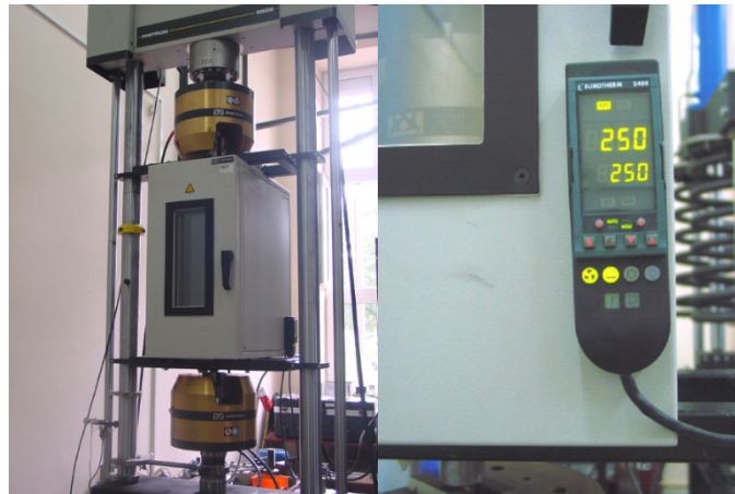
Fig. 2. Instron 8802 strength testing machine with climatic chamber Instron 3119-406-222
