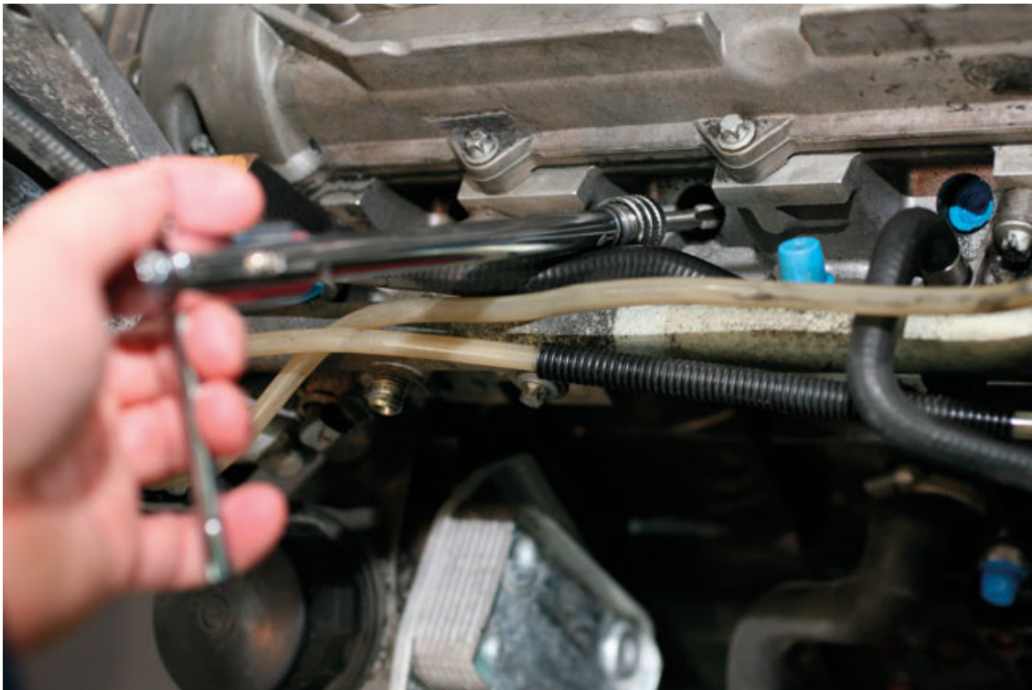
Fig. 3. Replacing spark plugs, glow plugs, and injectors is much easier to perform than replacing piston elements
