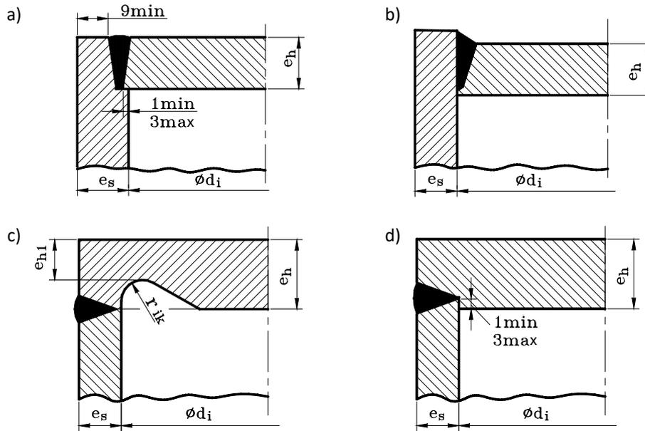
Fig. 1. Four recommended by EN 12952:3 designs for flat ends of boilers
