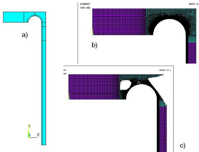
Fig. 4. Topological optimization of the studied boiler; (a) the basic structure, (b) area (finite elements) to modify (remove) marked in blue, (c) final result of the topological modification
