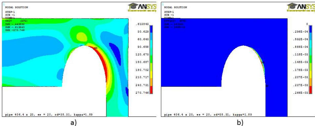
Fig. 3. Equivalent stress (a) and equivalent plastic strains distribution (b) for optimal parameters of stress relief groove of elliptic shape
