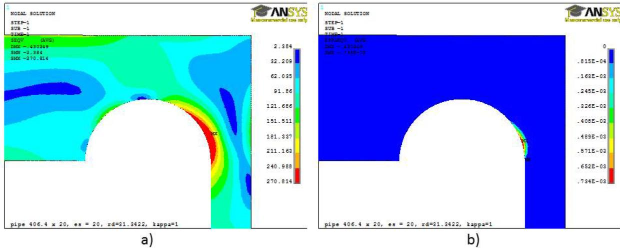
Fig. 2. Equivalent stress (a) and equivalent plastic strains distribution (b) for optimal parameters of stress relief groove of circular shape
