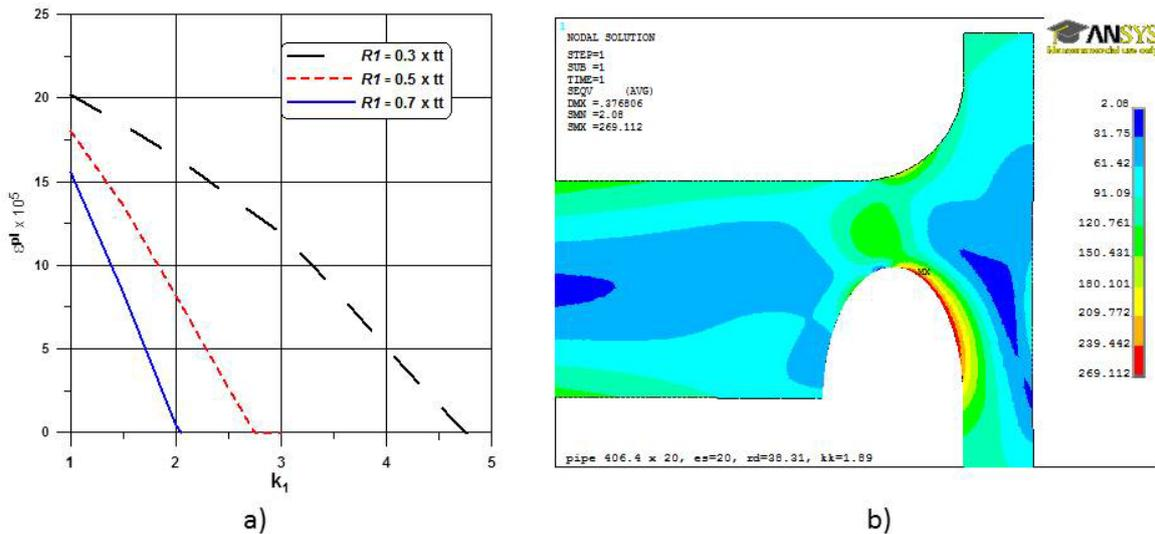
Fig. 7. Results of Concept 1 study: (a) maximum plastic deformation in analysed structure for different values of radius  $R1$  for concave face of weld and different height of band; (b) distribution of equivalent stress for  $R1 = 0.7 \times tt$  and  $hh = 2.05 \times es$
