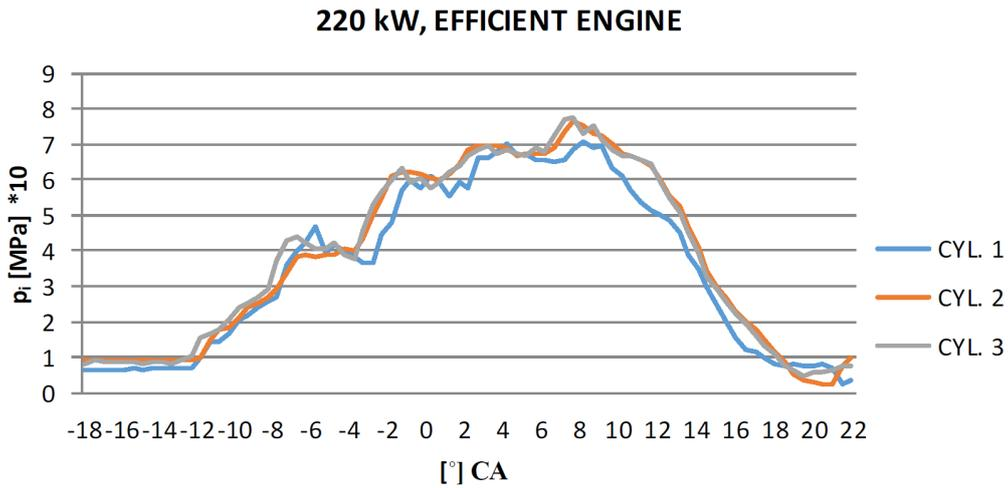
Fig. 8. Course of injection pressure curves at a given 220 kW load and standard engine operation
