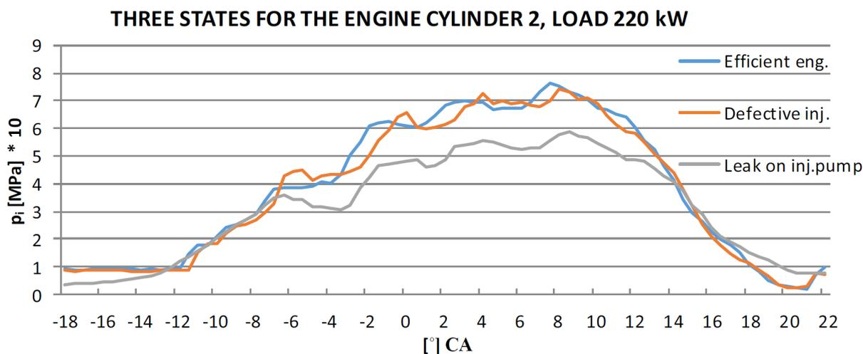
Fig. 11. Fuel injection pressure at 220 kW for cylinder number two. Comparison of effective engine injection pressure waveforms, leakage simulation on injection pump and simulation of faulty injector
