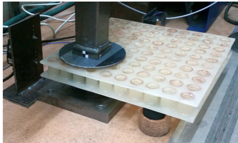
Fig. 3. Elastomer structure installed on the bench of the falling hammer
