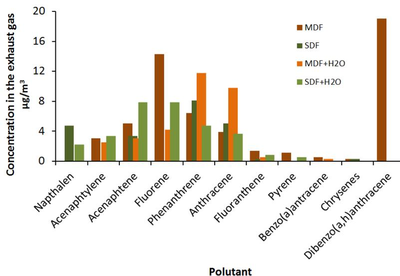
Fig. 3. Illustration of concentrations of emitted aromatic hydrocarbons (PAH) when engine is fuelled by different fuels
