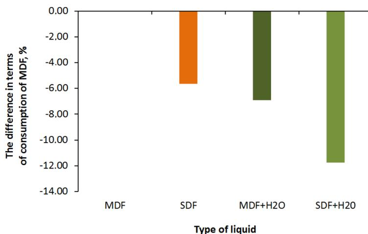
Fig. 2. Difference in fuel consumption with respect to mineral oil consumption
