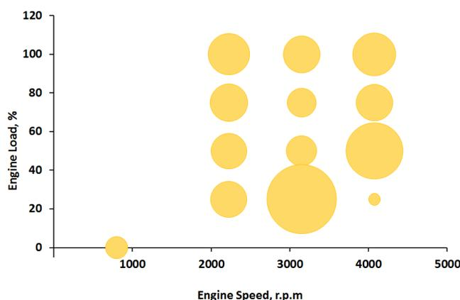
Fig. 1. Points motor characteristics corresponding to the requirements of the ESC test
