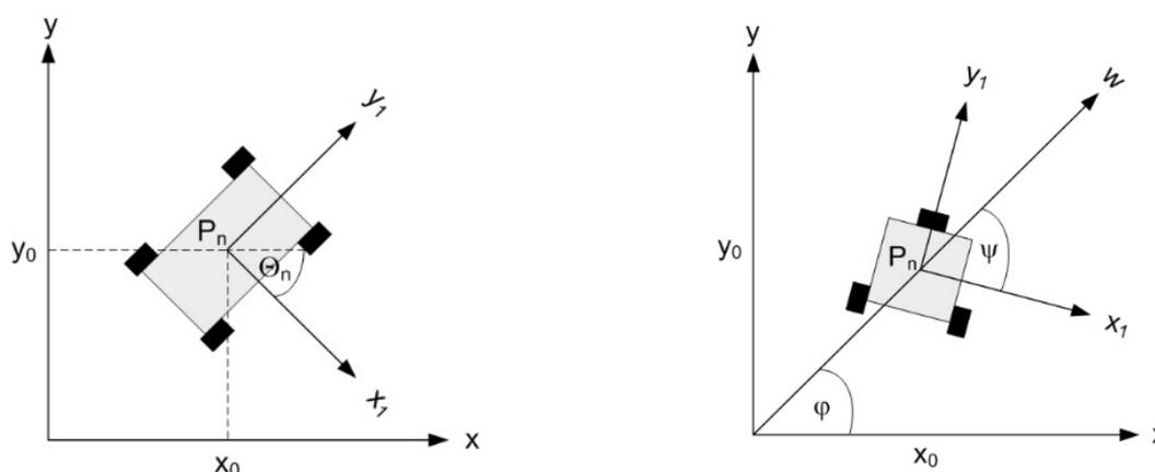
Fig. 2. From the left: nonholonomic kinematic structure (Fig. 2a), with holonomic kinematic structure (Fig. 2b)
