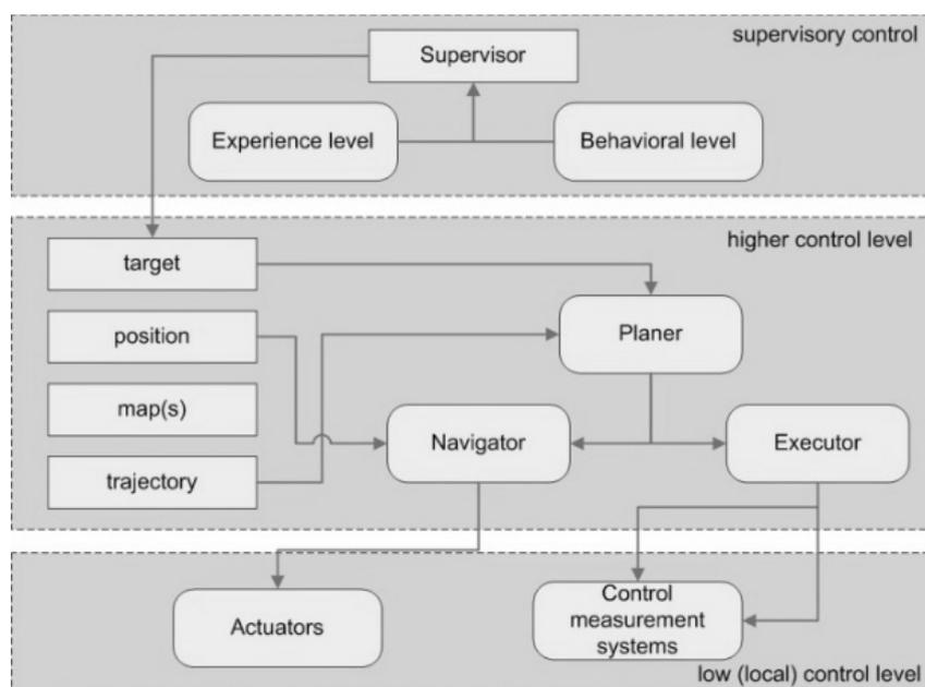
Fig. 3. The decentralized control system dedicated for AGV vehicles [18]
