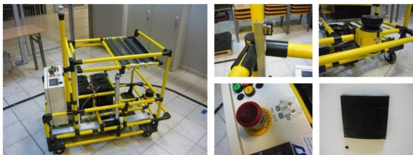
*Fig. 1. The AGV modular construction type*
