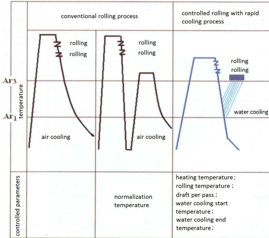
Fig. 1. Comparison of rolling processes [7]
