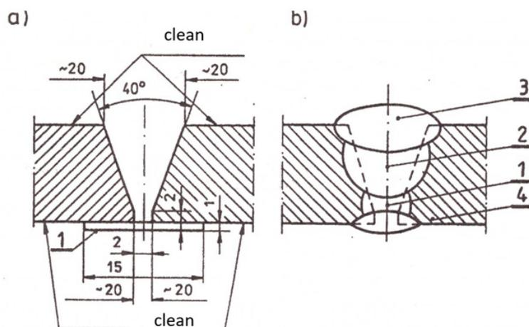
Fig. 3. The scheme of welding: a) sheets edges preparation: 1 – copper pad, b) welding sequence: 1 – before penetration run, 2 – filling run, 3 – closing run
