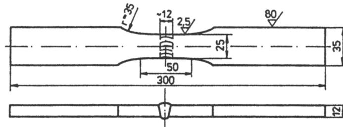
Fig. 4. Samples used for fatigue tests with weld nob's left in place
