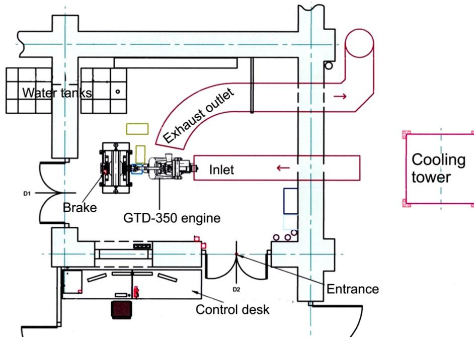
Fig. 2. GTD-350 test bench scheme
