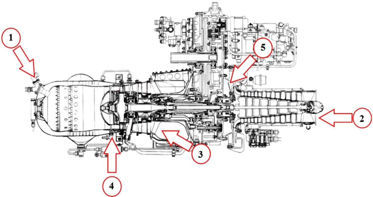
Fig. 9. GTD-350 cross-section with borescope entrances (1-5) [18]
