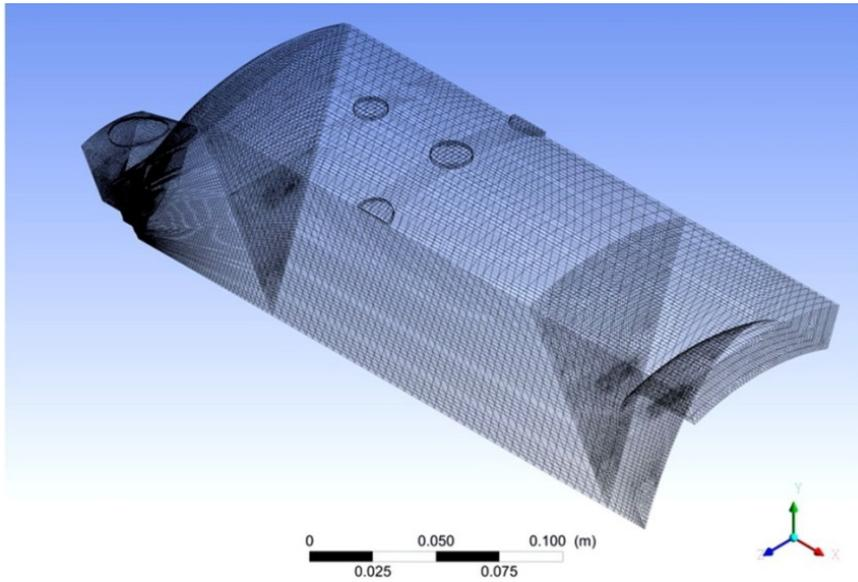
Fig. 3. Computational grid with hexahedral elements
