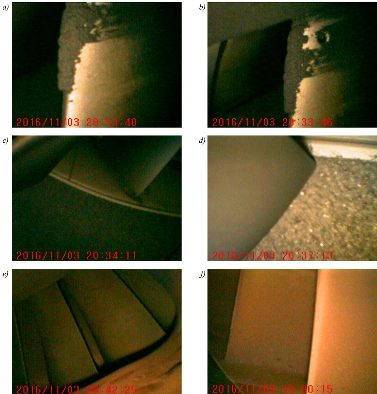
Fig. 14. GTD-350 compressor (a-d) and power turbine blades (e, f)
