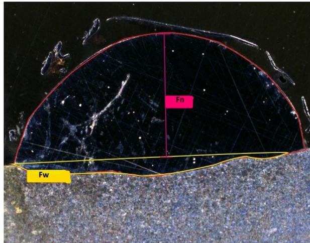
Fig. 1. Method of determination part of substrate material in padding weld of the test sample
