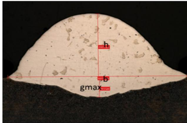
Fig. 2. The dimensions of padding weld geometry
