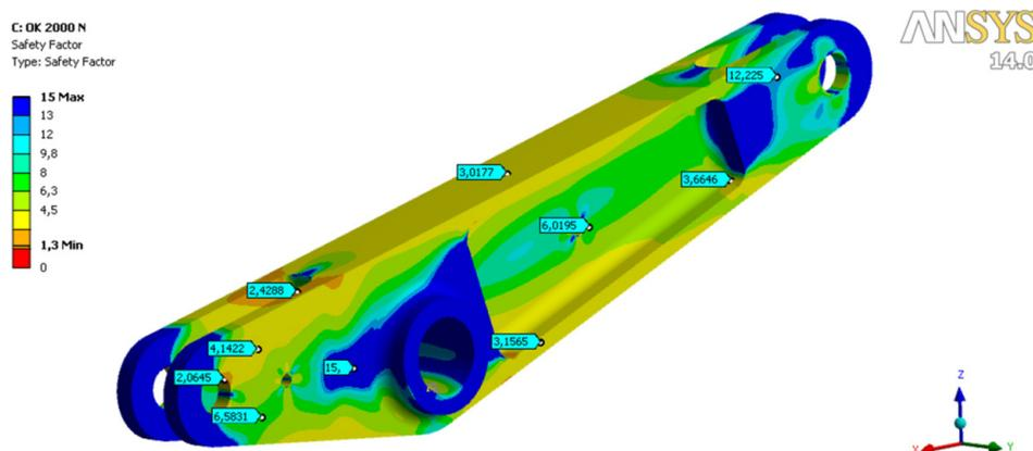
Fig. 5. Distribution of the safety factor on the control – system lever
