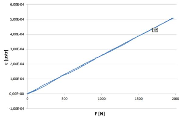
Fig. 8. Deformation values for loads 2000 N, reading of the unidirectional strain gauge T2
