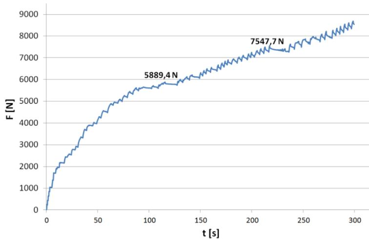
Fig. 10. Force value during time of the destruction test
