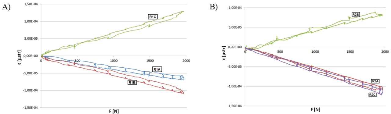
Fig. 9. Deformation values for loads 2000 N, reading of the strain rosette A – R1, B – R2
