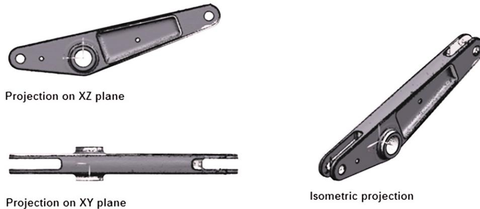
Fig. 2. Projection on plane superimposed: CAD model (light grey) and measuring object (dark grey)
