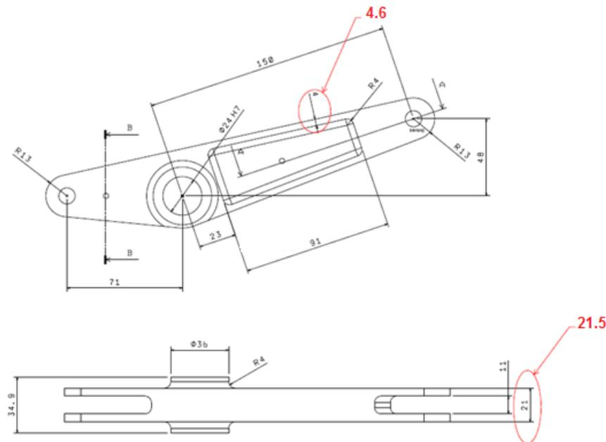
Fig. 3. The most visible changes in the magnesium alloy control – system lever geometry
