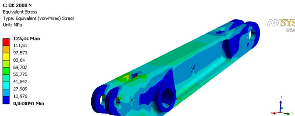
Fig. 4. Stress distribution of the control – system lever
