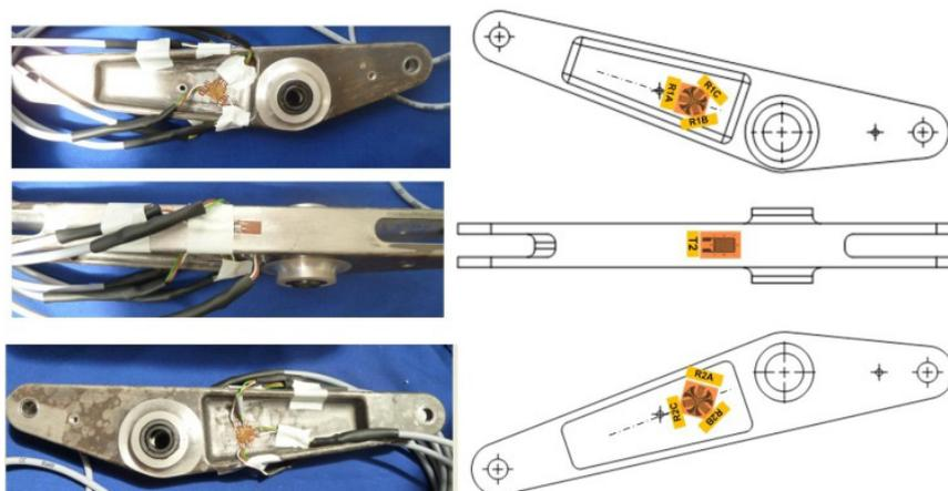
Fig. 7. Strain gauge points installation
