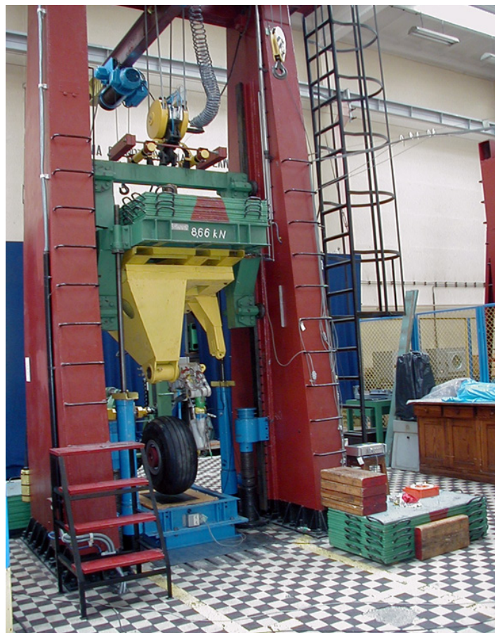
Fig. 5. Free fall dynamic drop test machine example, Note the ground plate below the landing gear, source ILot
