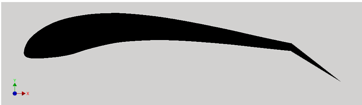
Fig. 2. NACA M8 airfoil with plain flaps ( 30^\circ )
