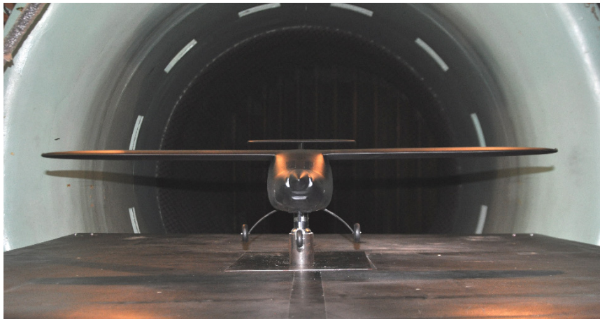
Fig. 2. Model of the ultralight aircraft mounted in the test section of the T-1 low speed wind tunnel
