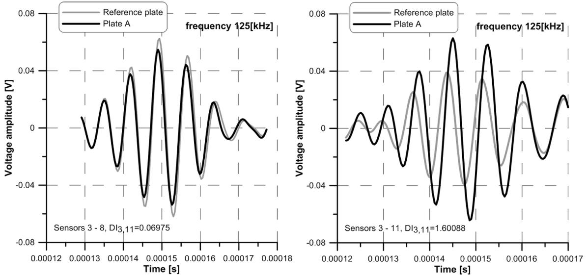
Fig. 5. Comparison of the anti-symmetric A0 modes for intact and damaged structure
