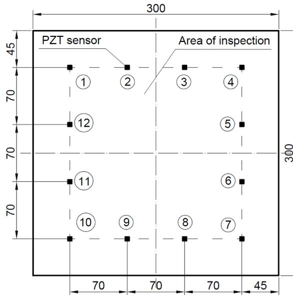
Fig. 1. Investigated hybrid composite plate with network of PZT sensors
