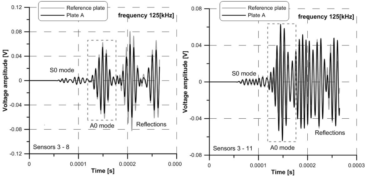
Fig. 4. Comparison of obtained signals in the case of following pair of sensors 3-8 and 3-11
