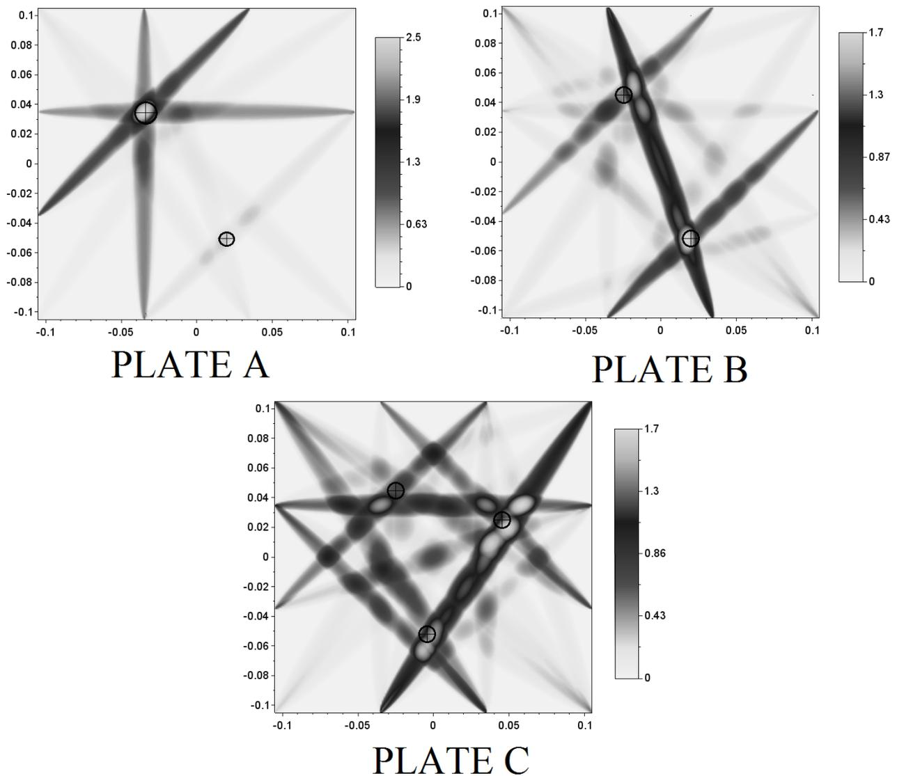
*Fig. 7. Localization of damages in the case of plate A, B and C*
