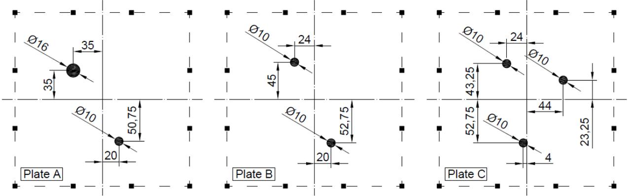
Fig. 3. Localizations of damages in studied structures
