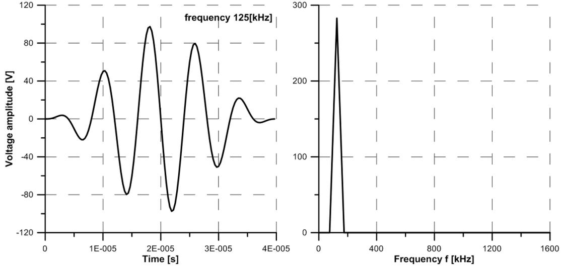
Fig. 2. Excitation signal in time and frequency domain
