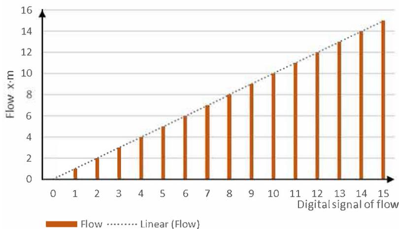
Fig. 3. Characteristic of flow through the binary control valve
