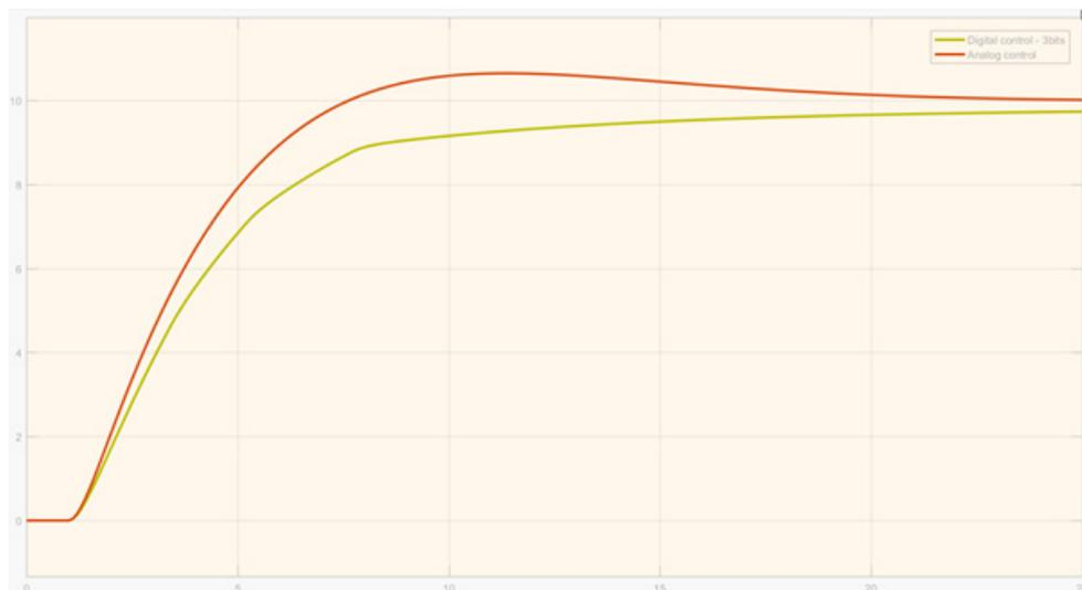
Fig. 5. Comparing the response in continuous control and binary control in a simulated example
