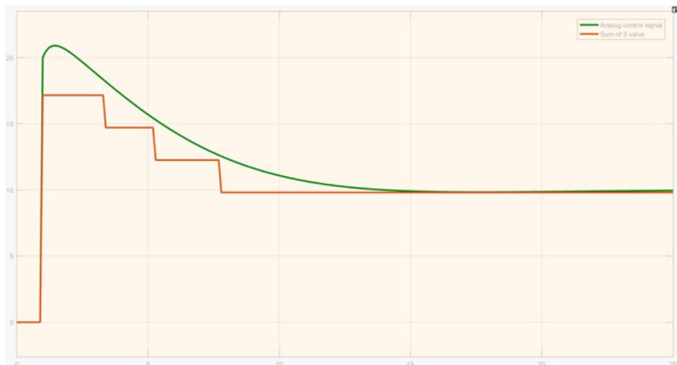
Fig. 6. Comparing the error signal in continuous control and binary control in a simulated example
