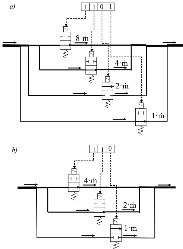
Fig. 1. Diagram of the control valve, a – four bits, b – three bits
