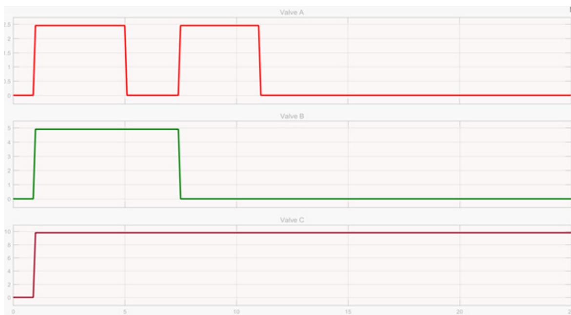
Fig. 7. The extracted bits of signals in a simulated example: A – work time of first valve, B – work time of second valve, C – work time of third valve
