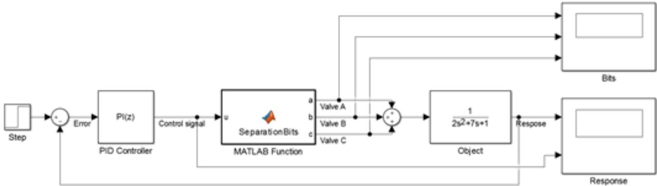
Fig. 4. The project simulation of control in MATLAB Simulink
